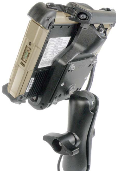
Figure 25. X10gx Vehicle Dock on a Ball Mount Assembly
