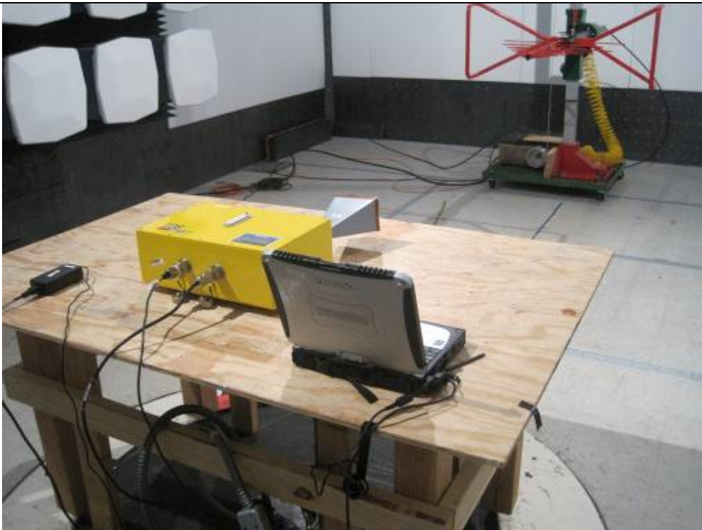
Radiated Emission Test Setup(22dBi Antenna) – Rear View
