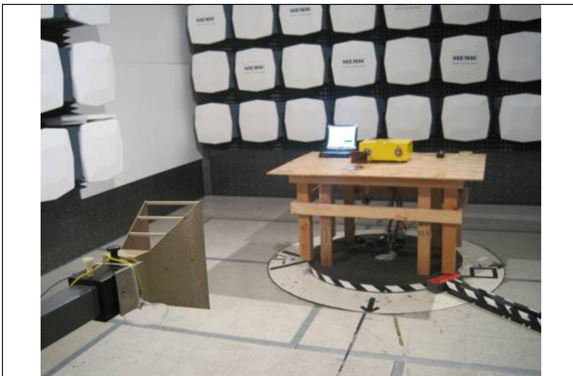
Radiated Emission Test Setup(22dBi Antenna) – Front View
