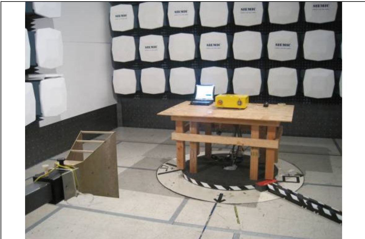
Radiated Emission Test Setup(15dBi Antenna) – Front View
