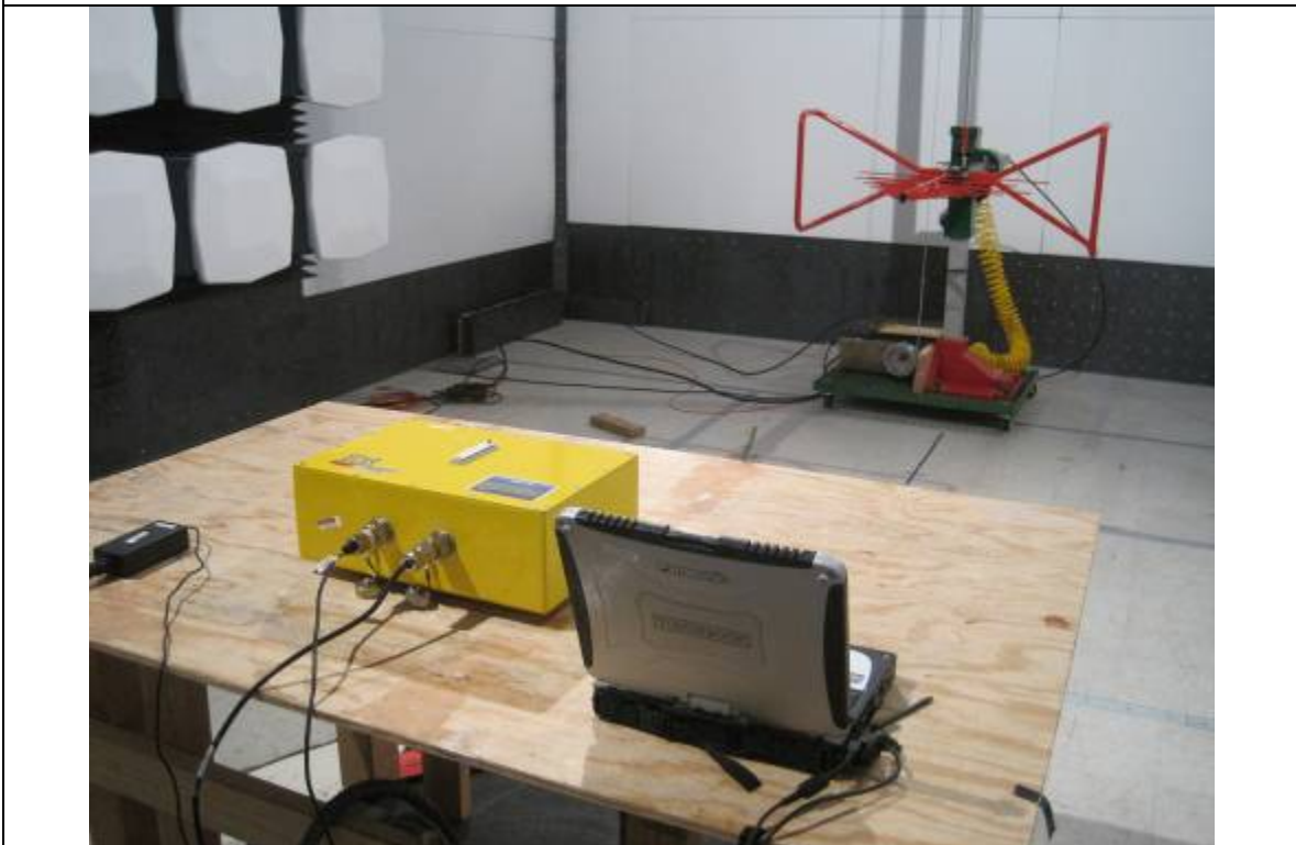
Radiated Emission Test Setup(15dBi Antenna) – Rear View
