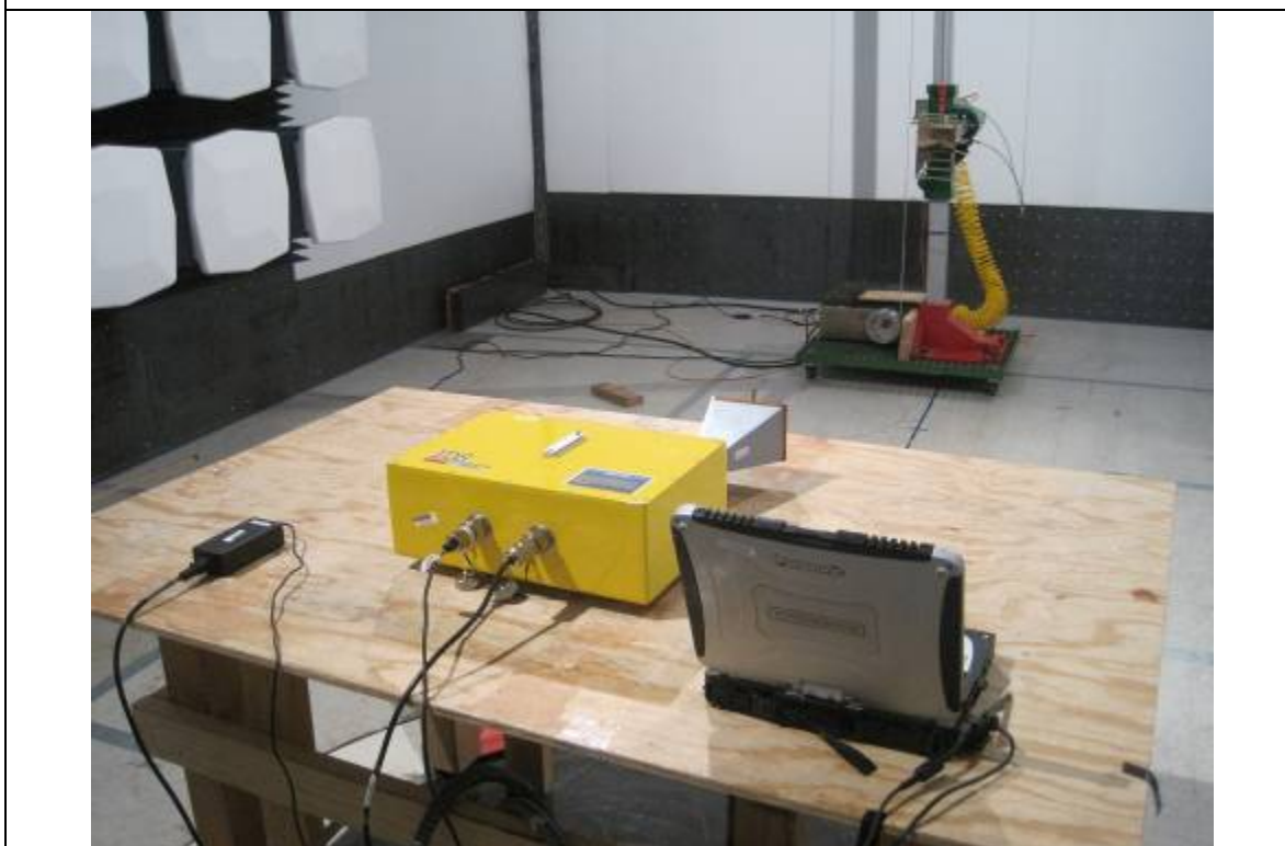
Radiated Emission Test Setup(22dBi Antenna) – Rear View
