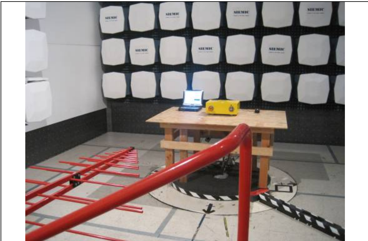
Radiated Emission Test Setup(15dBi Antenna) – Front View
