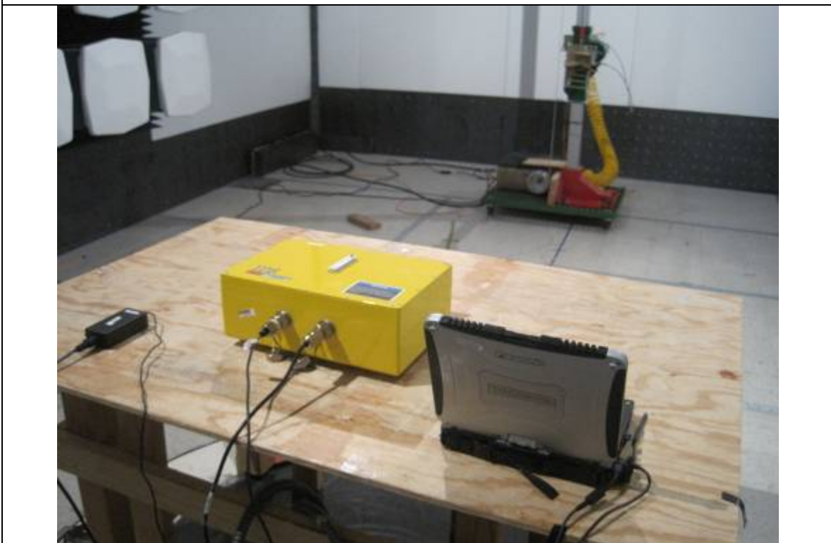
Radiated Emission Test Setup(15dBi Antenna) – Rear View
