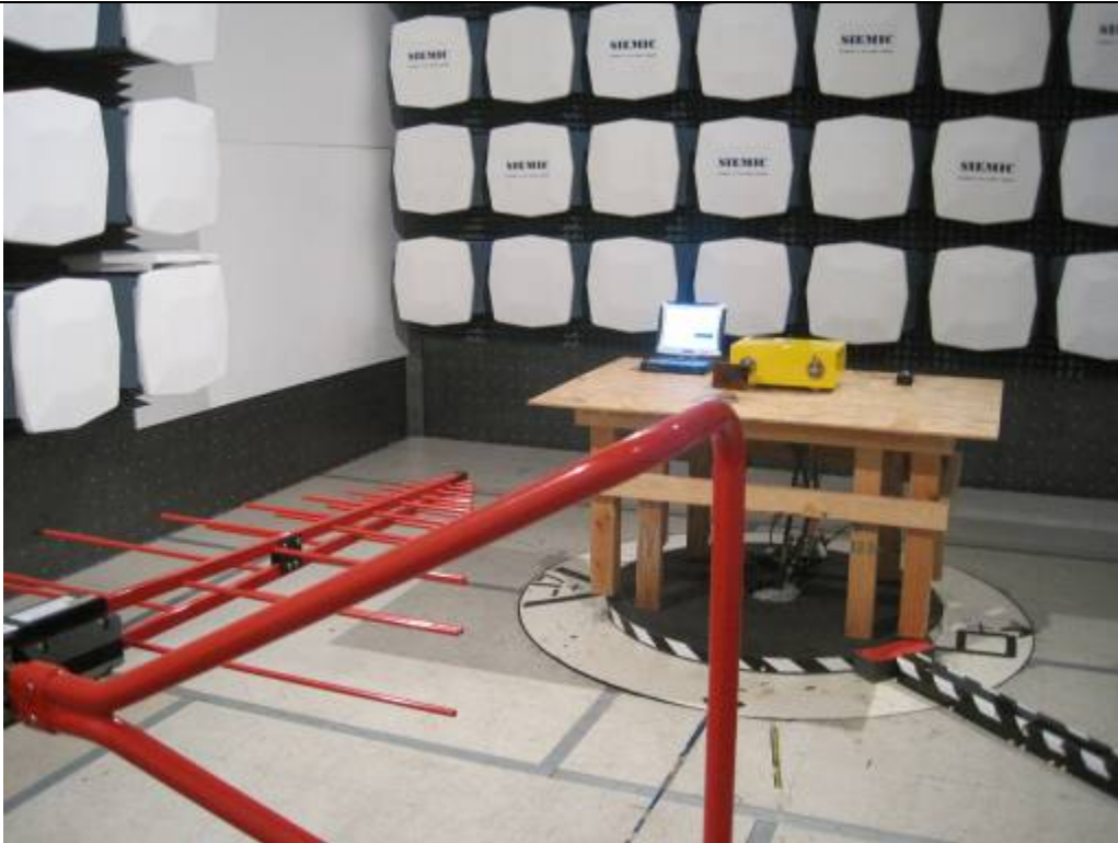
Radiated Emission Test Setup (22dBi Antenna) - Front View
