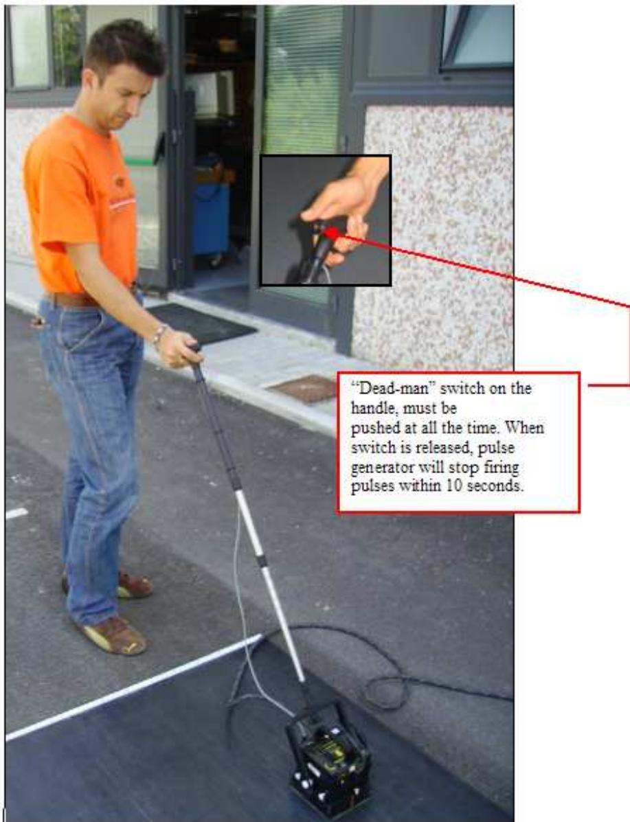
"Dead-man" switch on the handle, must be pushed at all the time. When switch is released, pulse generator will stop firing pulses within 10 seconds.
