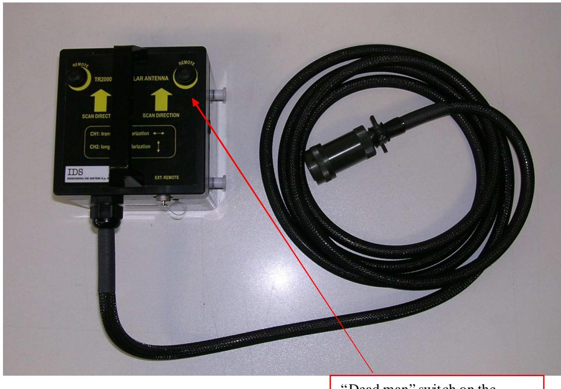
“Dead-man” switch on the antenna, must be pushed at all time. When switch is released, pulse generator will stop firing pulses within 10 seconds.
