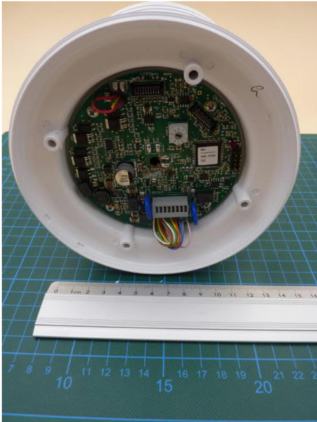
WS600-UMB housing with main PCB, shielding removed
