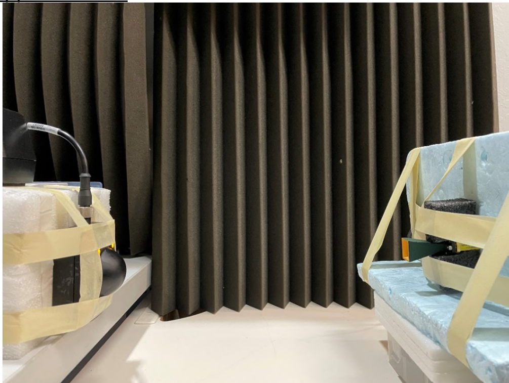
Photo 6: Test setup for step 1: measuring the main beam of the EUT with RF detector and DSO.
