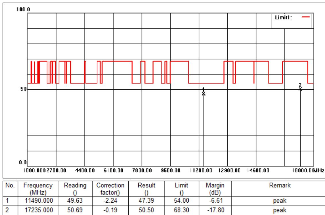
Mode:d; Polarization:Vertical; Modulation:c; bandwidth:20MHz; Channel:Low
