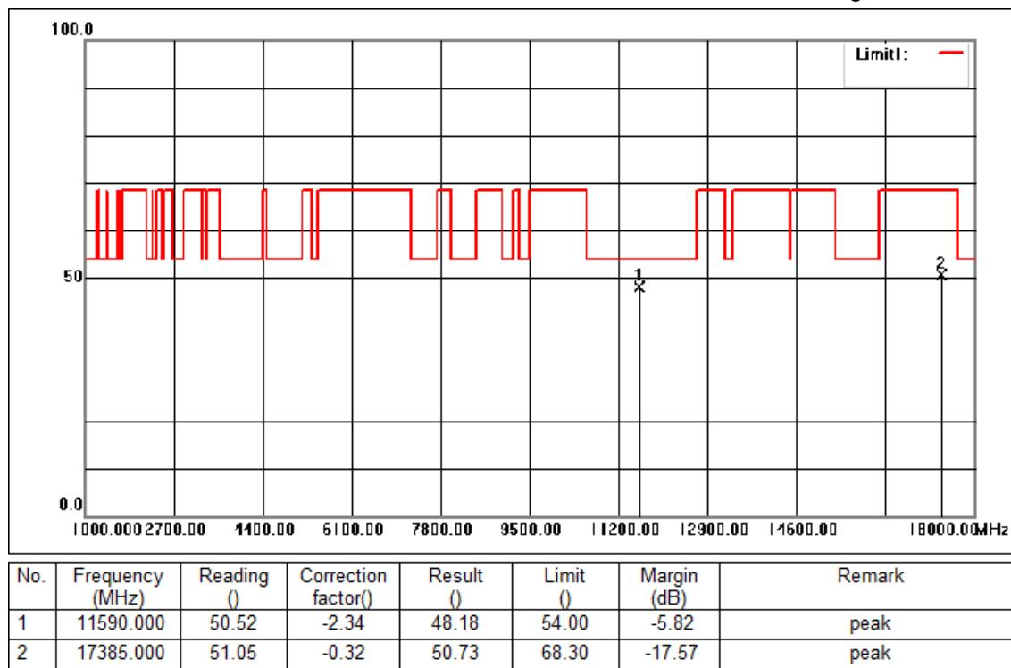
Mode:d; Polarization:Vertical; Modulation:c; bandwidth:40MHz; Channel:High
