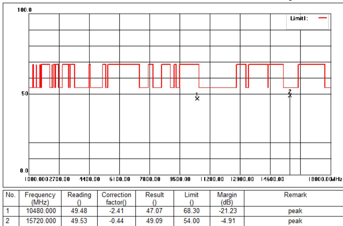
Mode:c; Polarization:Vertical; Modulation:a; bandwidth:20MHz; Channel:High
