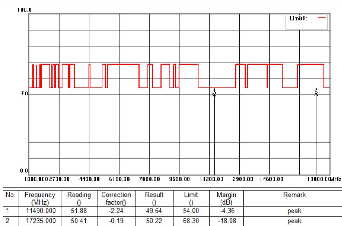
Mode:d; Polarization:Horizontal; Modulation:n; bandwidth:20MHz; Channel:middle
