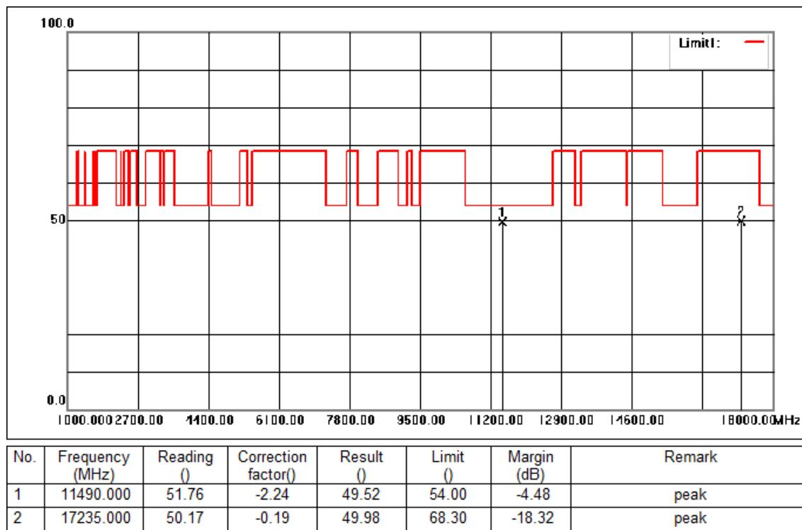
Mode:d; Polarization:Vertical; Modulation:a; bandwidth:20MHz; Channel:Low
