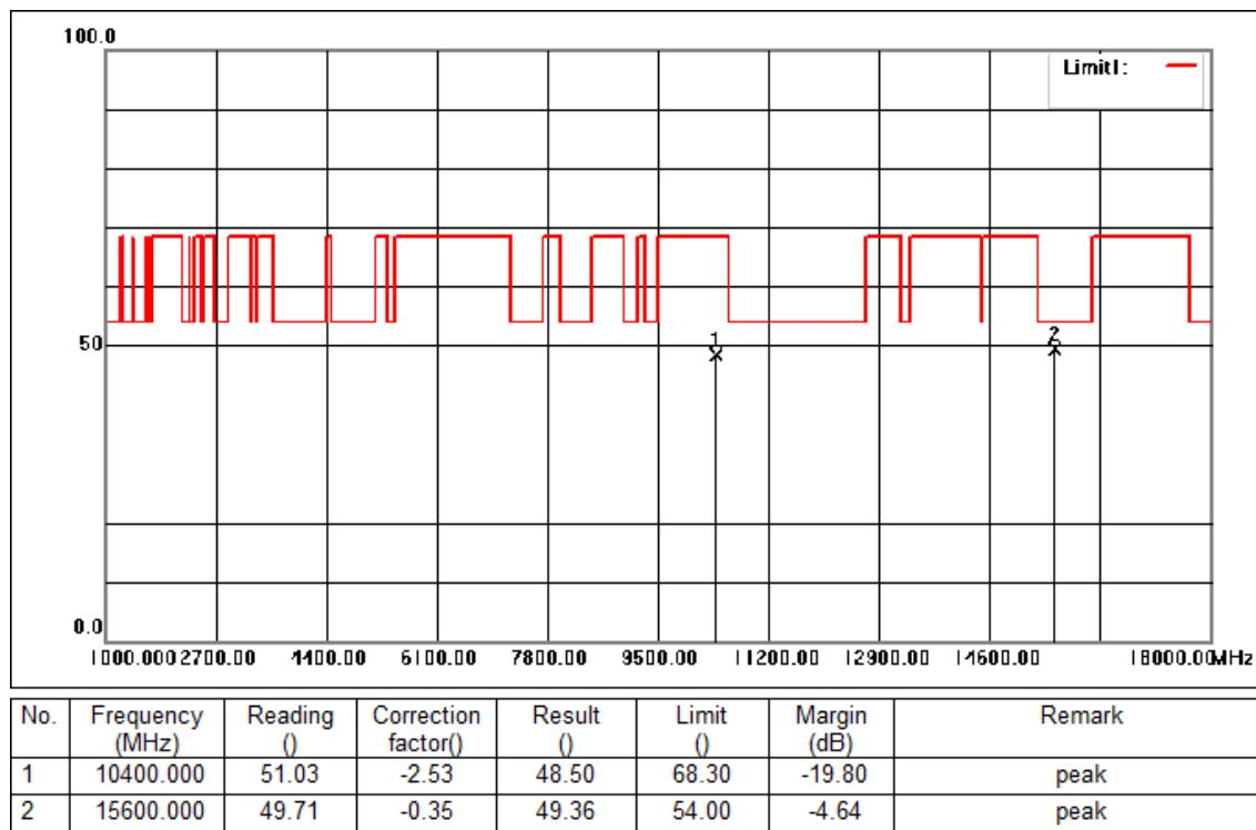
Mode:c; Polarization:Vertical; Modulation:n; bandwidth:20MHz; Channel:middle
