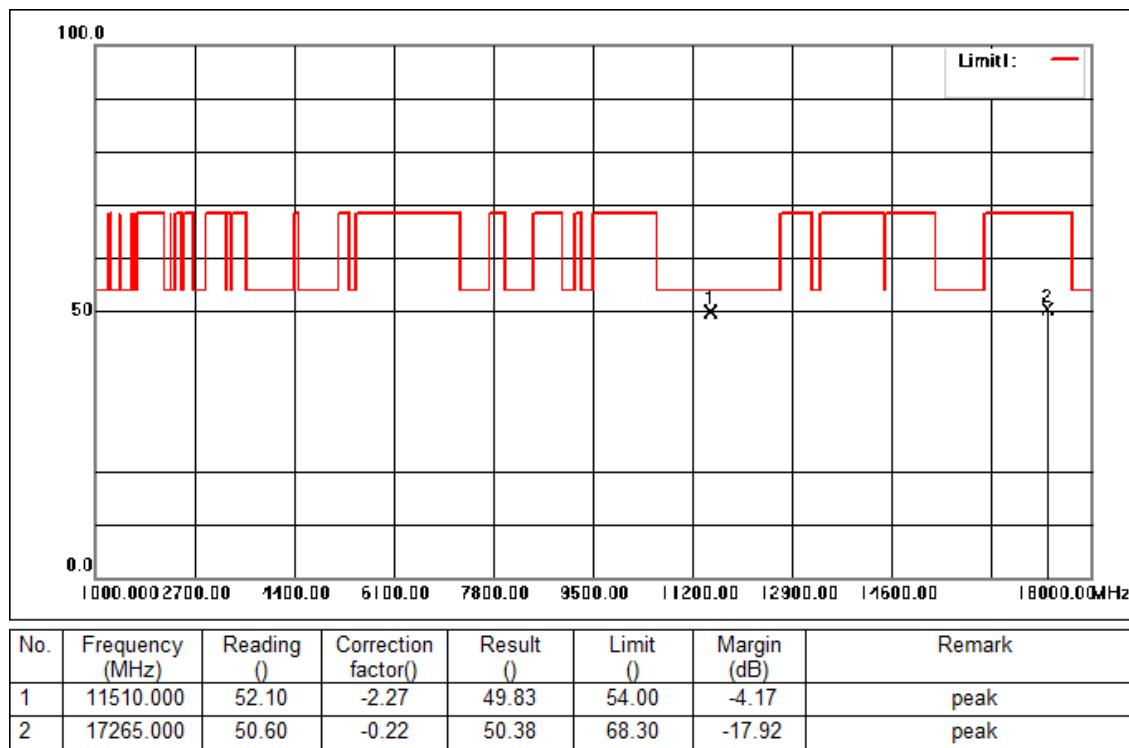
Mode:d; Polarization:Horizontal; Modulation:n; bandwidth:40MHz; Channel:High
