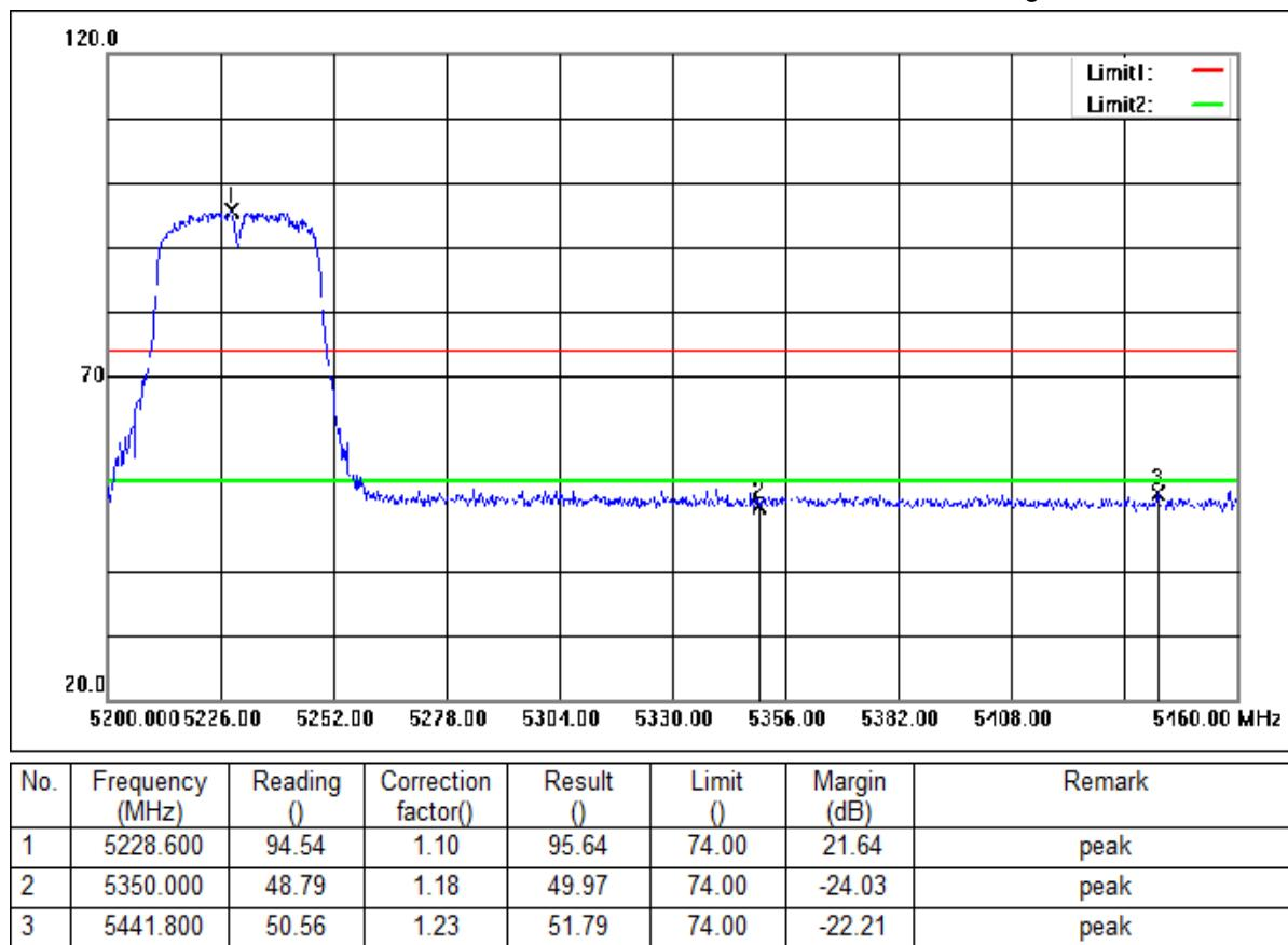
Mode:c; Polarization:Vertical; Modulation:c; bandwidth:40MHz; Channel:High
