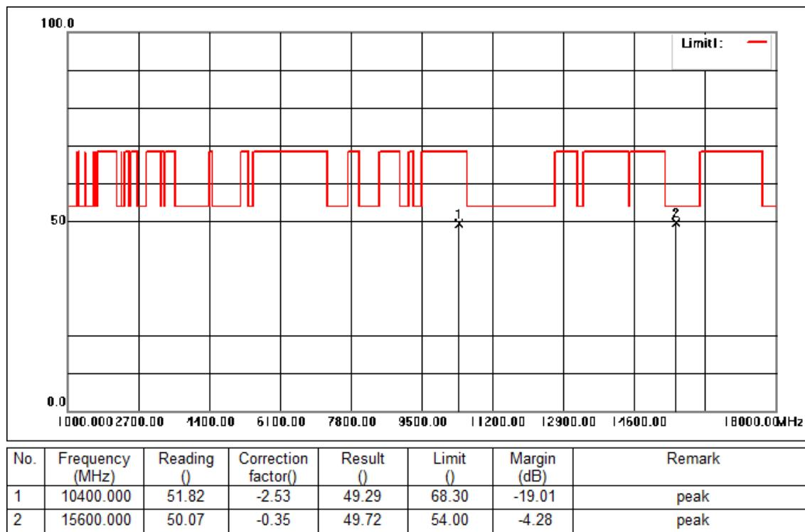
Mode:c; Polarization:Horizontal; Modulation:c; bandwidth:20MHz; Channel:High
