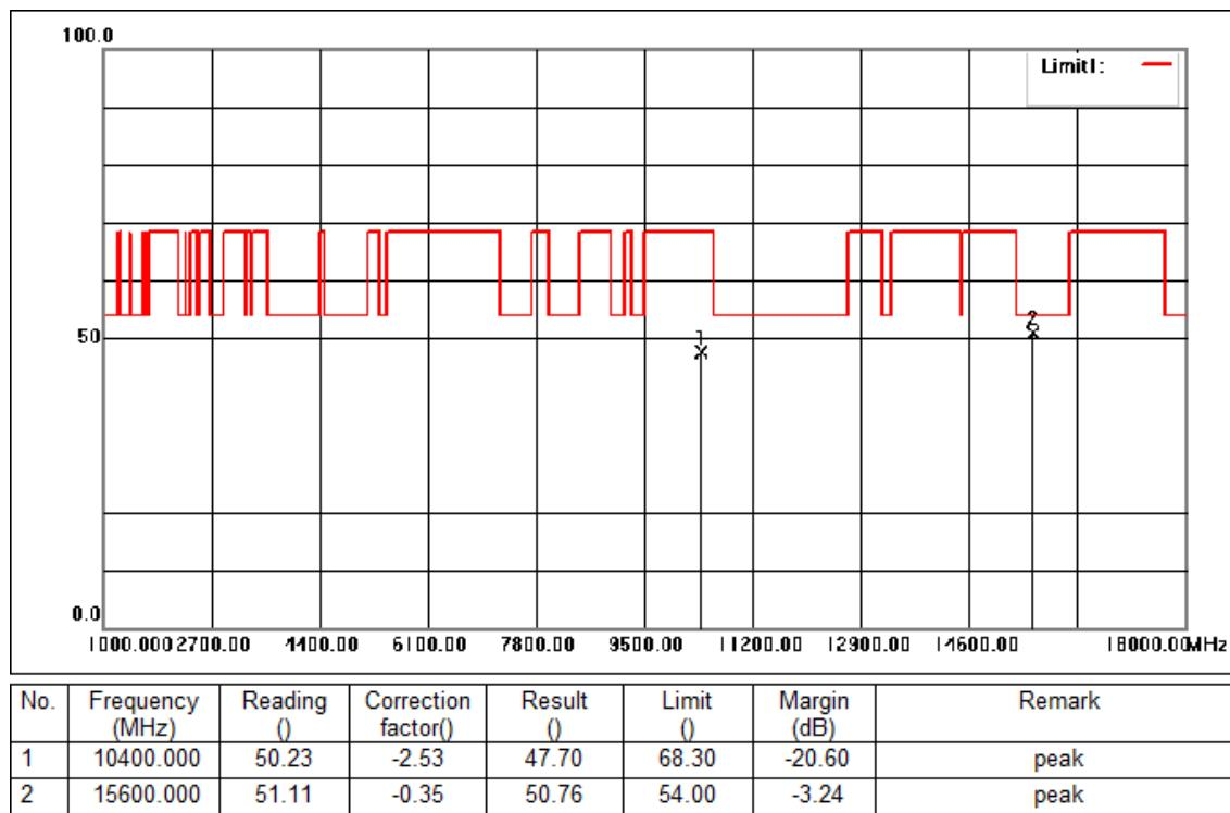
Mode:c; Polarization:Vertical; Modulation:a; bandwidth:20MHz; Channel:middle
