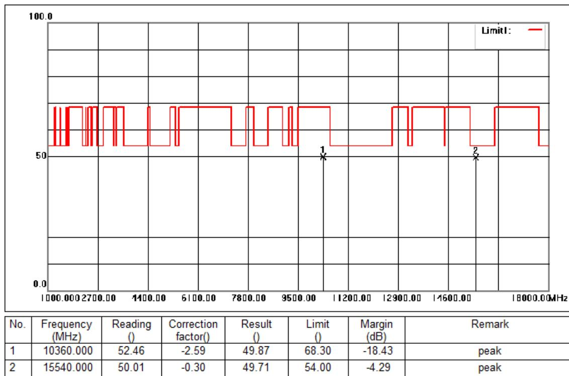
Mode:c; Polarization:Vertical; Modulation:c; bandwidth:20MHz; Channel:Low
