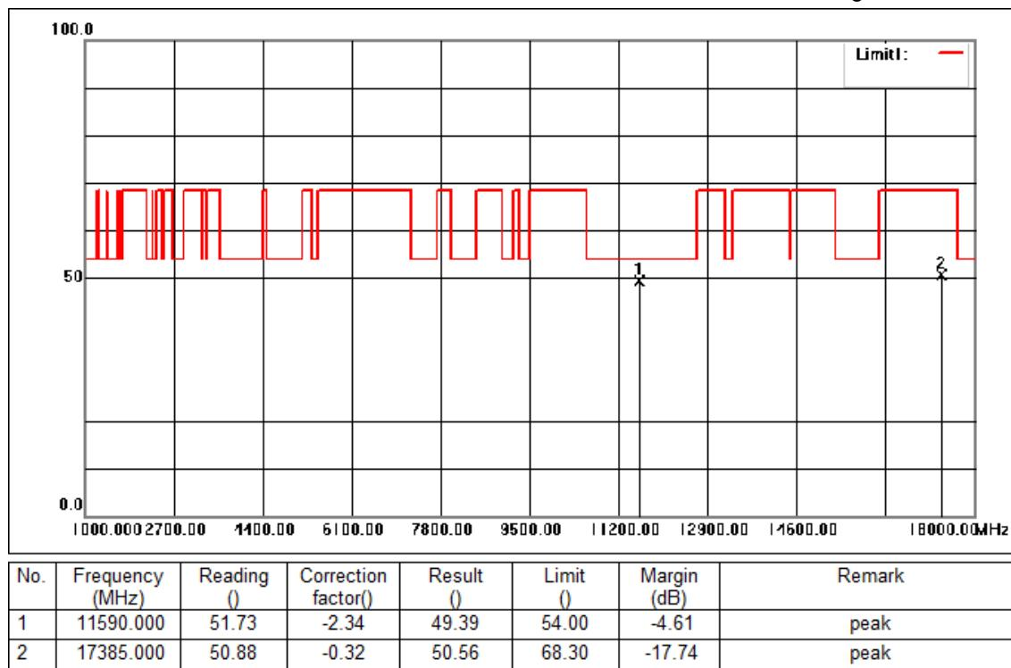
Mode:d; Polarization:Vertical; Modulation:n; bandwidth:40MHz; Channel:High
