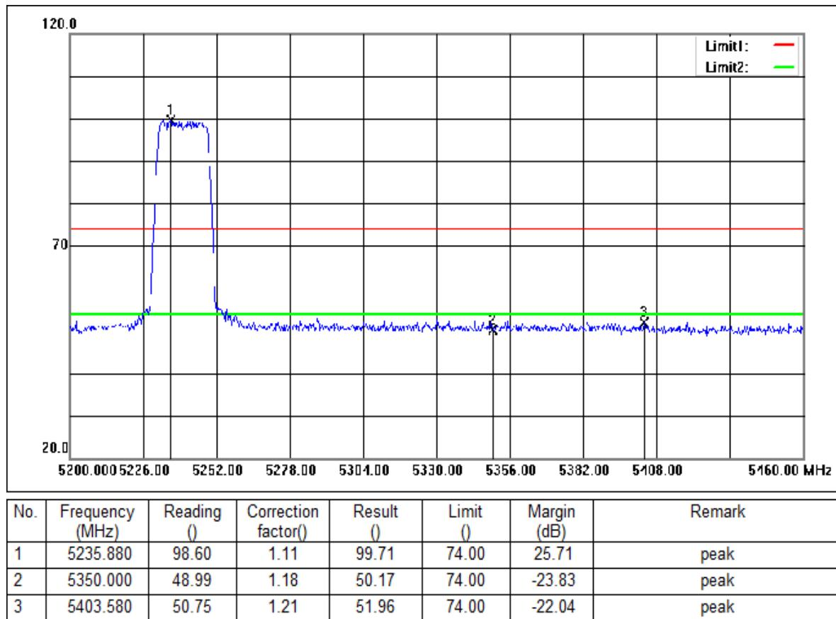
Mode:c; Polarization:Vertical; Modulation:n; bandwidth:20MHz; Channel:High
