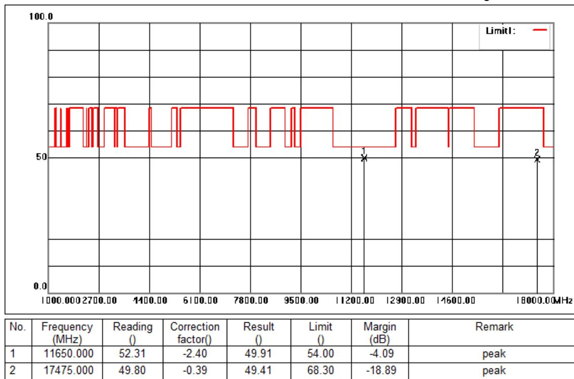
Mode:d; Polarization:Vertical; Modulation:n; bandwidth:20MHz; Channel:High
