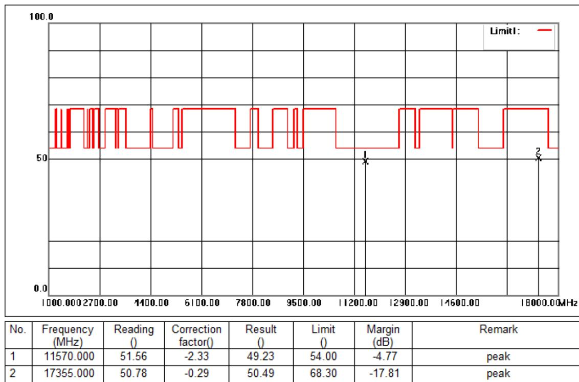
Mode:d; Polarization:Vertical; Modulation:c; bandwidth:20MHz; Channel:middle
