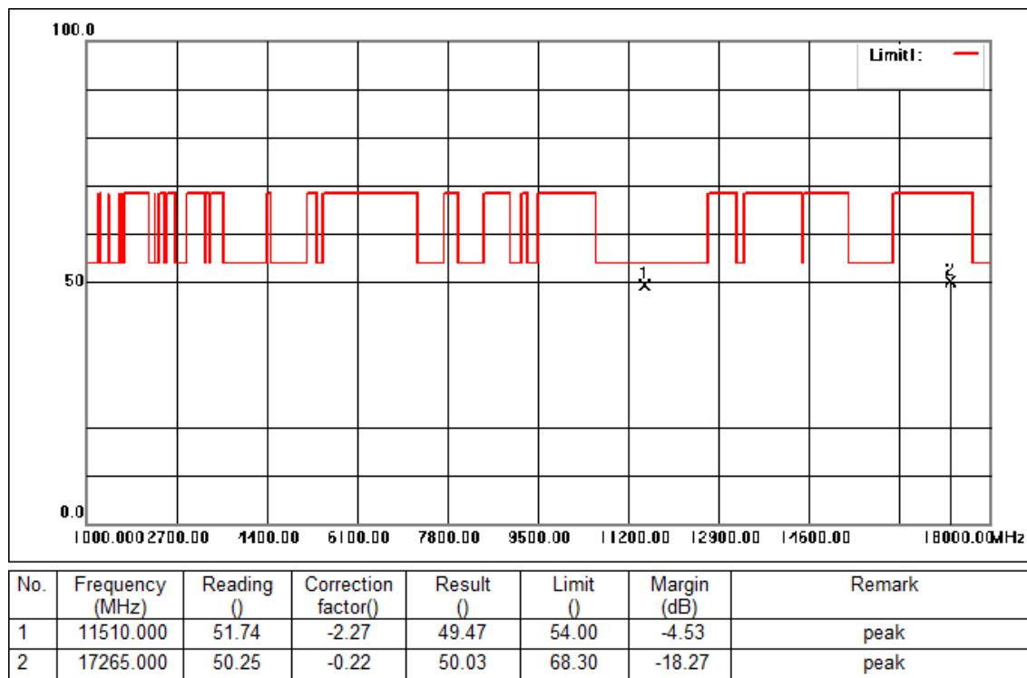
Mode:d; Polarization:Vertical; Modulation:n; bandwidth:40MHz; Channel:Low
