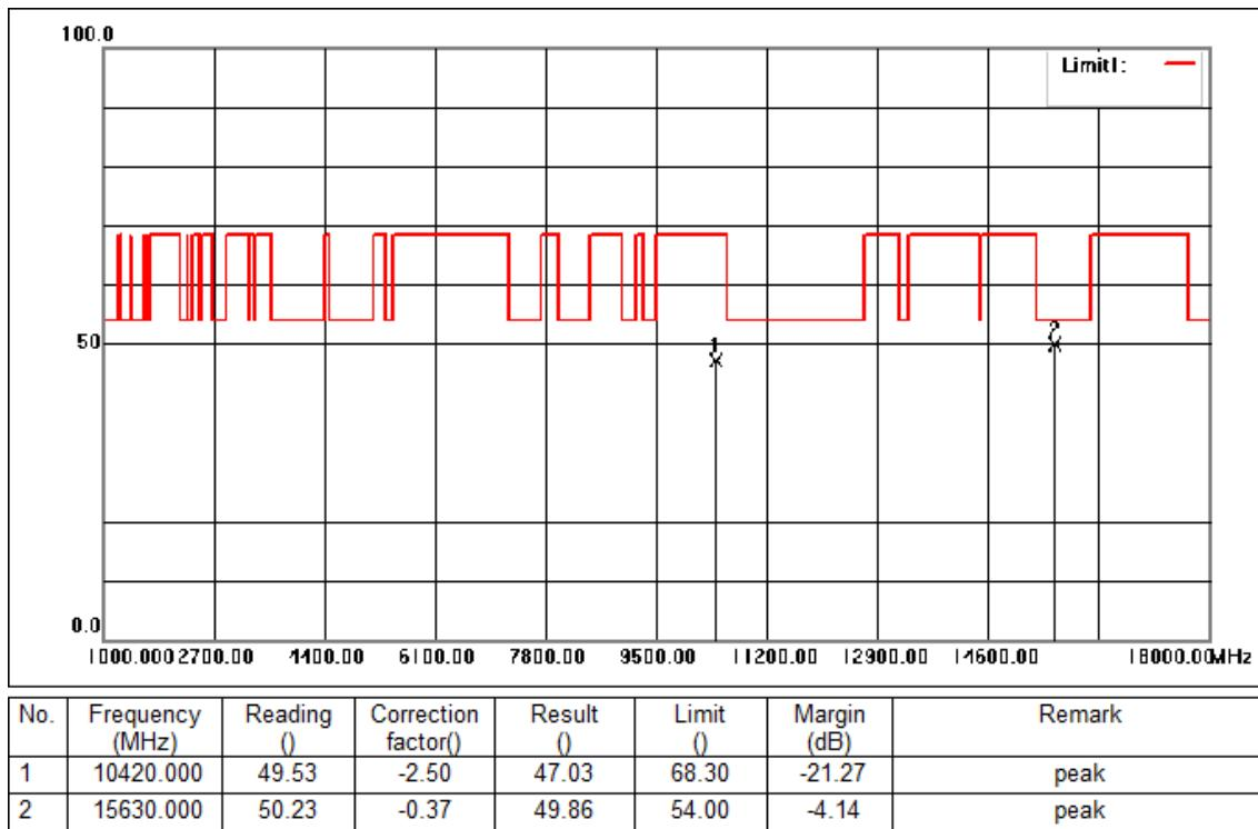
Mode:c; Polarization:Vertical; Modulation:c; bandwidth:80MHz; Channel:Low
