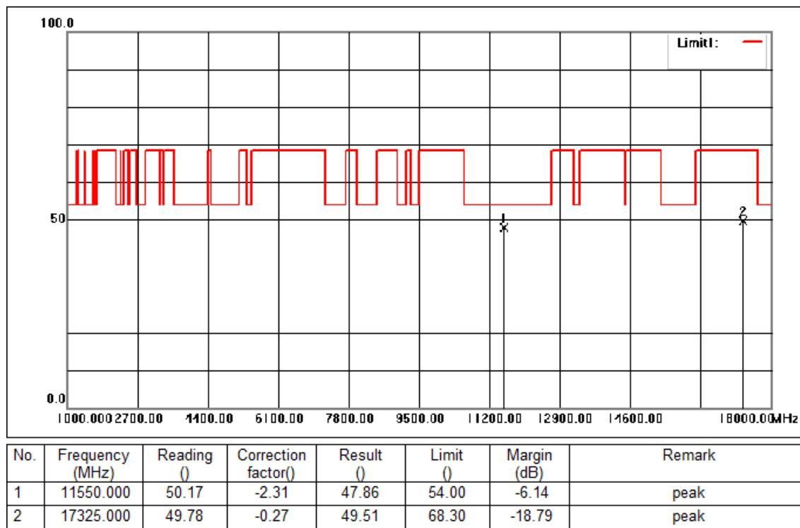
Mode:c; Polarization:Horizontal; Modulation:n; bandwidth:40MHz; Channel:High
