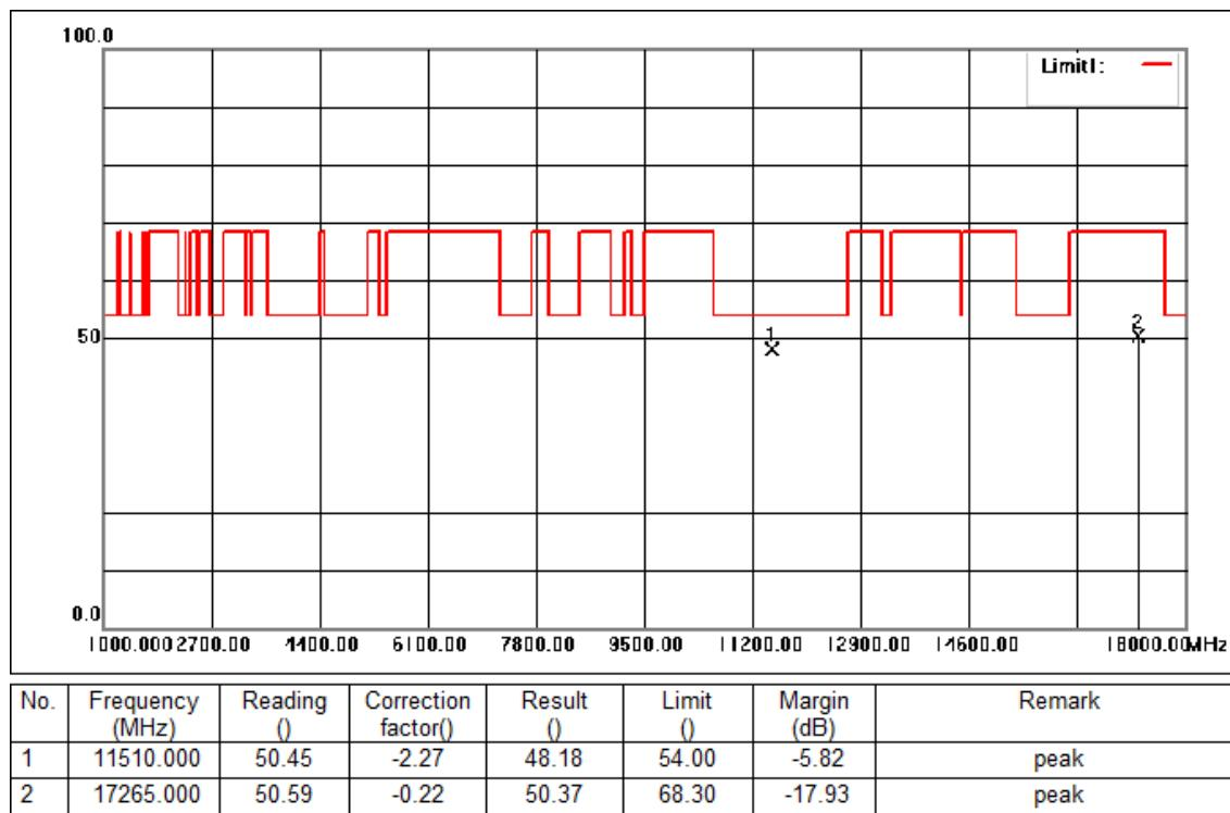
Mode:d; Polarization:Vertical; Modulation:c; bandwidth:40MHz; Channel:Low
