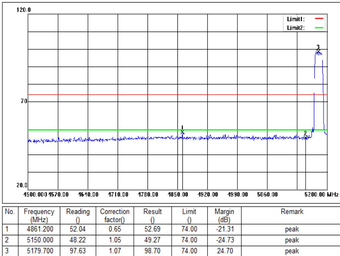
Mode:c; Polarization:Vertical; Modulation:n; bandwidth:20MHz; Channel:Low
