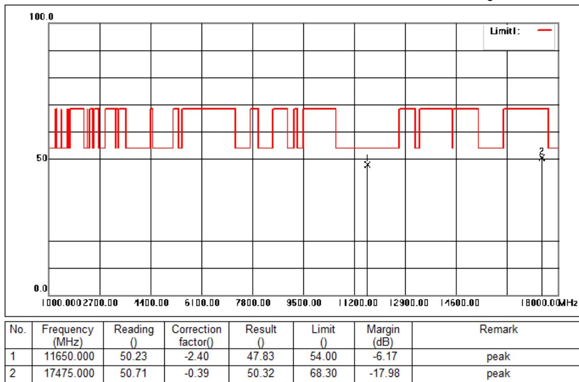
Mode:d; Polarization:Vertical; Modulation:c; bandwidth:20MHz; Channel:High
