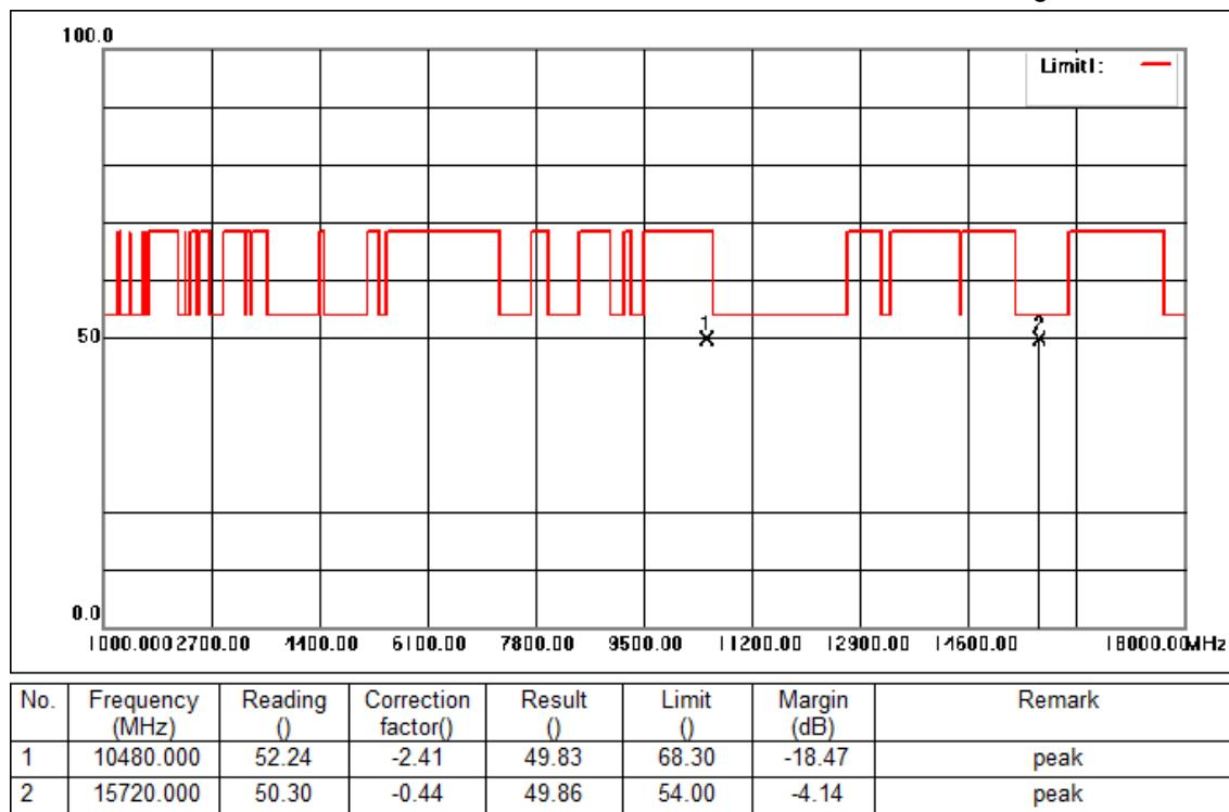
Mode:c; Polarization:Vertical; Modulation:n; bandwidth:20MHz; Channel:High
