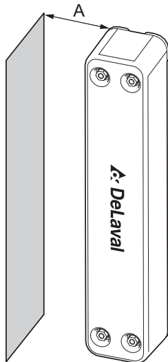
Fig. 5: IPR positioning near metal objects.
