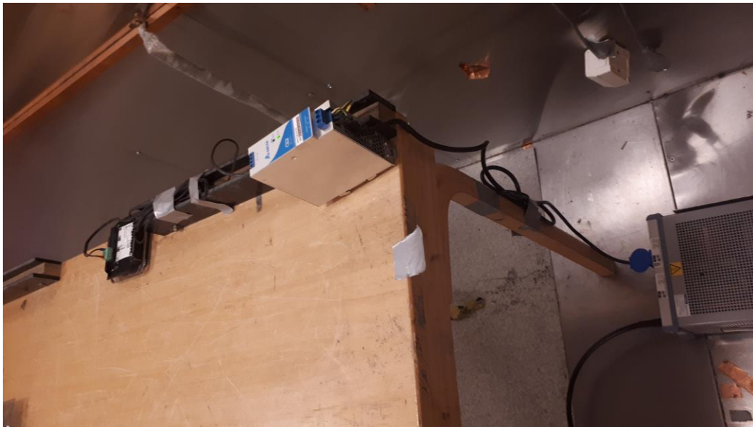
Conducted spurious emissions mains. EUT to the left and power supply to the right.
