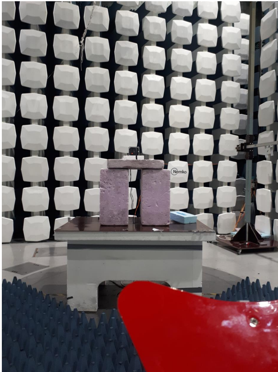
Radiated Spurious Emissions, 1 GHz – 18 GHz, as seen from antenna The antenna shown is the EMCO 3117PA antenna
