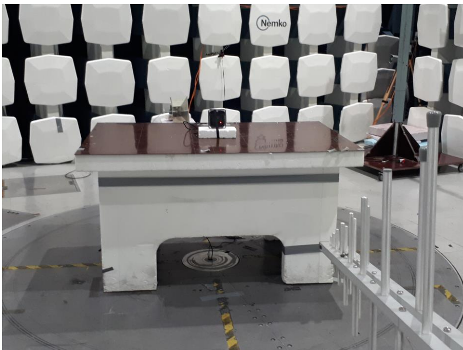
Radiated Emissions, 30 - 1000 MHz, as seen from antenna
