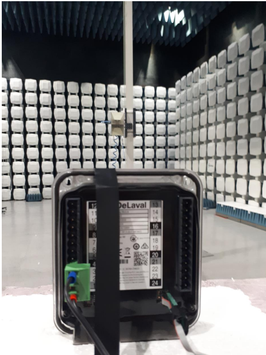
Radiated Emissions, 1 GHz – 18 GHz, as seen from EUT. The EMCO 3115 antenna (shown in picture) was used for eirp and Band Edge tests
