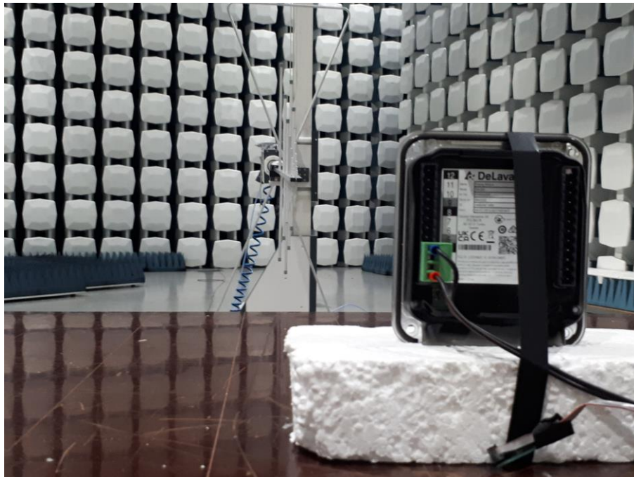
Radiated Emissions, 30 - 1000 MHz, as seen from EUT The cable in front is the programming cable from PC
