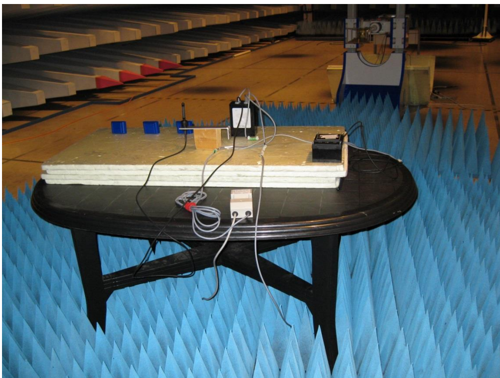
Photo 4.1.4 Test setup regarding measurement of radio frequency electromagnetic field > 1 GHz
