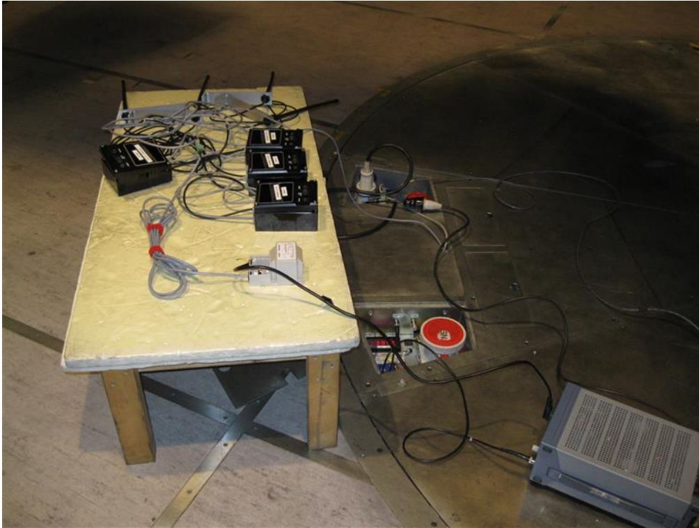
Photo 4.2.1 Test setup regarding measurement of radio frequency voltage on mains. Only 2 of 4 units powered.
