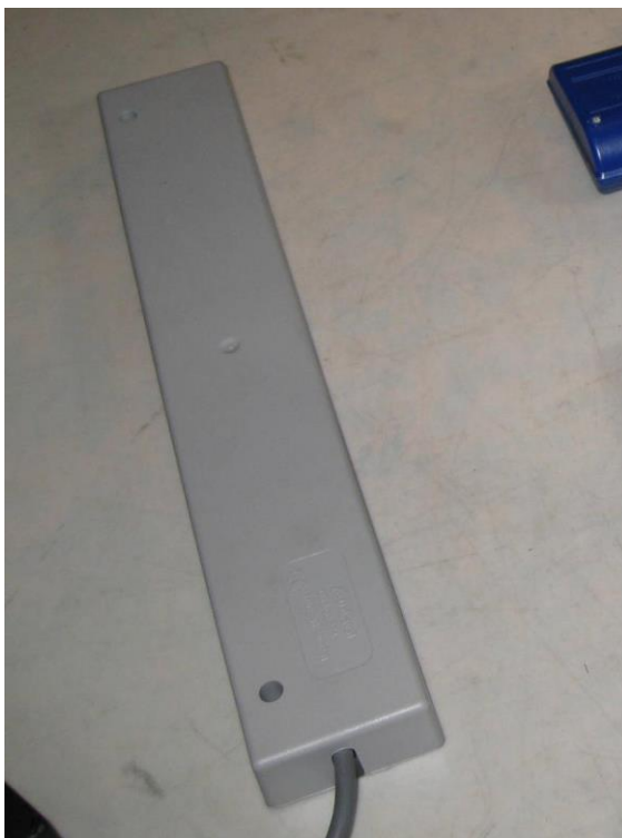
Photo 2.2.5 Auxiliary equipment. RFID reader.2.2.3.
