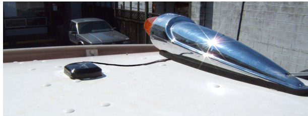
Figure 3-1 GPS antenna mounted on a roof and facing up to the sky
