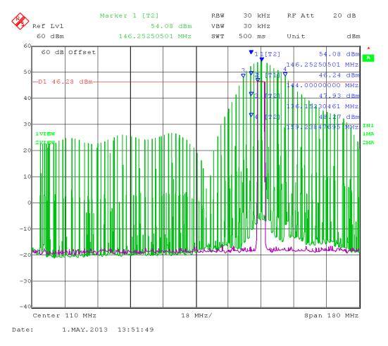
The output of the amplifier (green) has been plot from 20 to 200 MHz with the input level was steady at 46.28 dBm.
