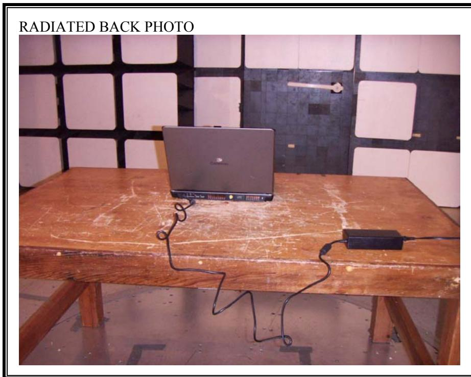
**POWERLINE CONDUCTED EMISSIONS MEASUREMENT SETUP**
