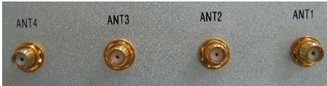
Figure2.4 - RFS2314 Antenna Connections
