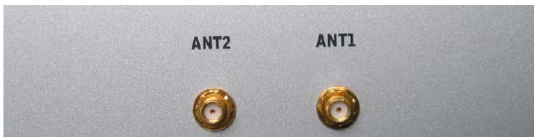
Figure 2.3 - RFS2312 Antenna Connections
