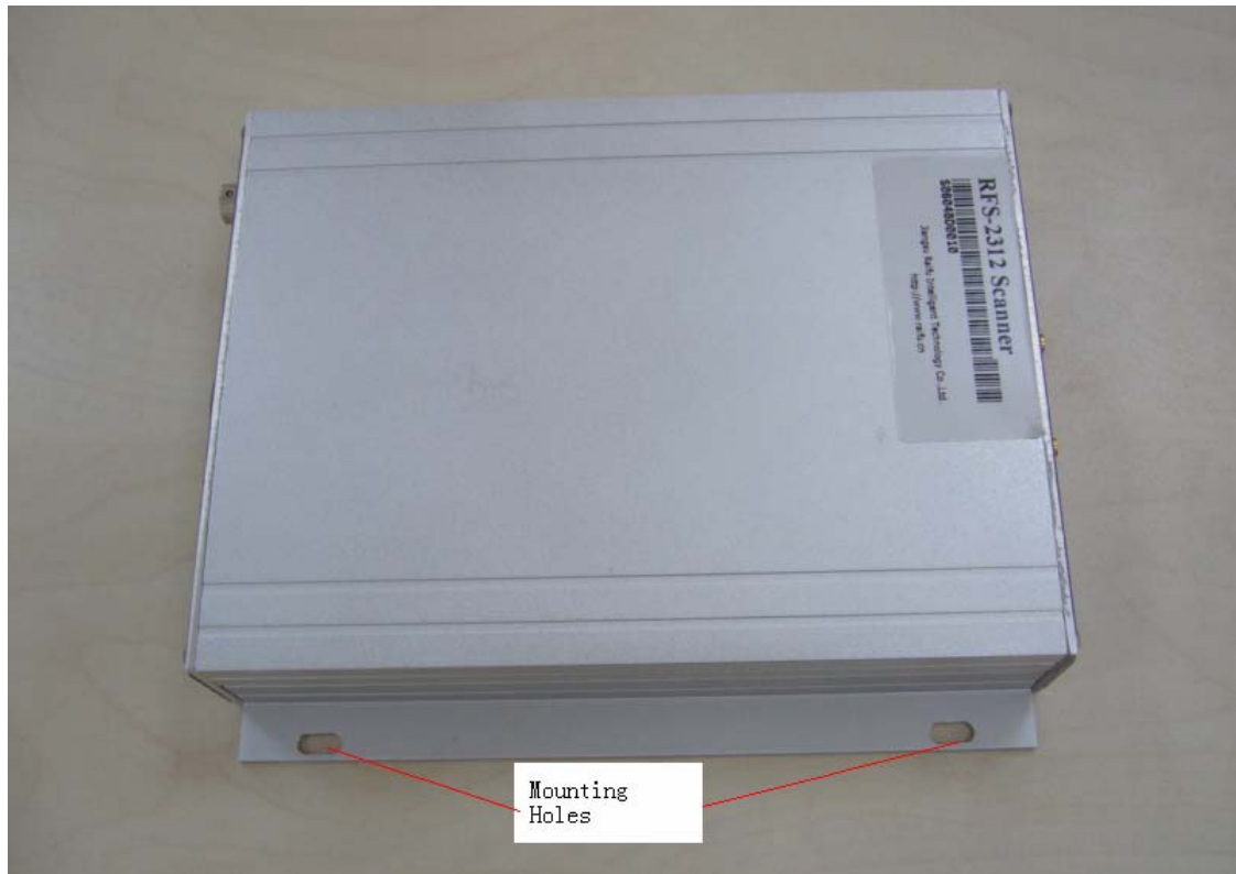
Figure 2.9 - View of the Reader showing mounting holes
