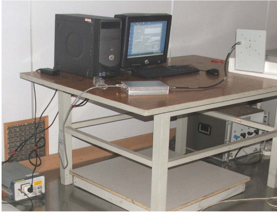
Conducted Emission Test Set-up - Front View
