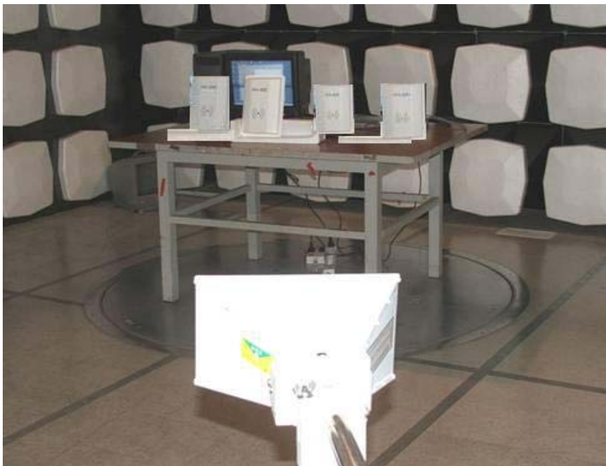
Radiated Emissions Test Set-up (Above 1GHz)
