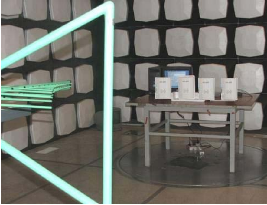
Radiated Emissions Test Set-up (Below 1GHz)
