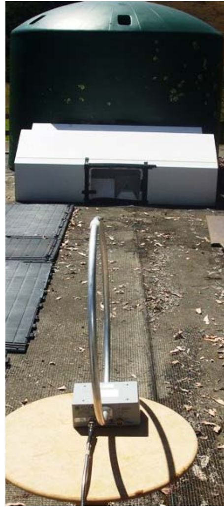
Test shed showing a loop antenna in use.
