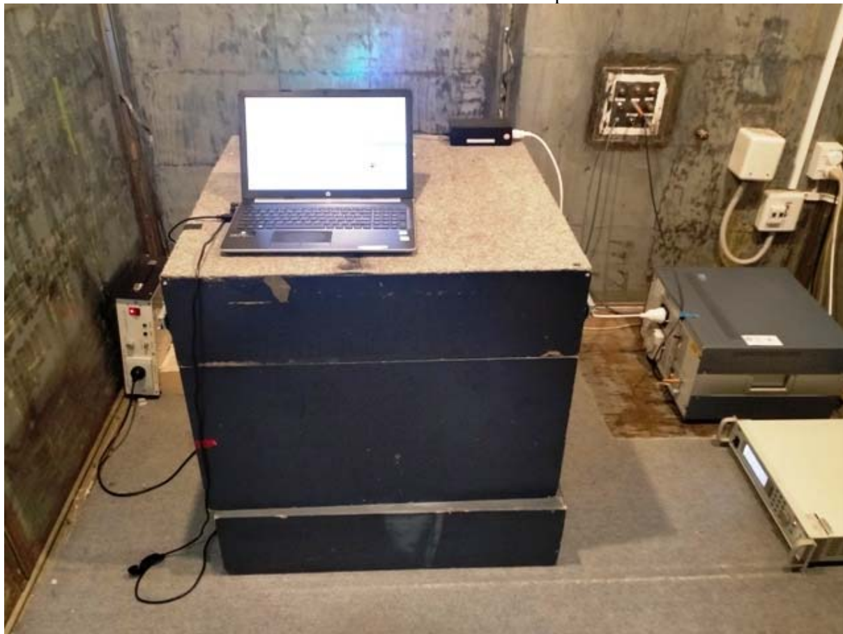
Conducted emissions test setup
