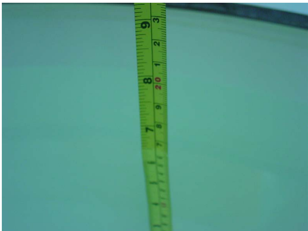
Picture B2: Liquid depth in the Flat Phantom (PCS 1900MHz)
