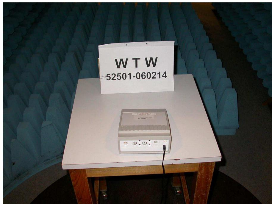
**Test setup for radiated emission measurement
