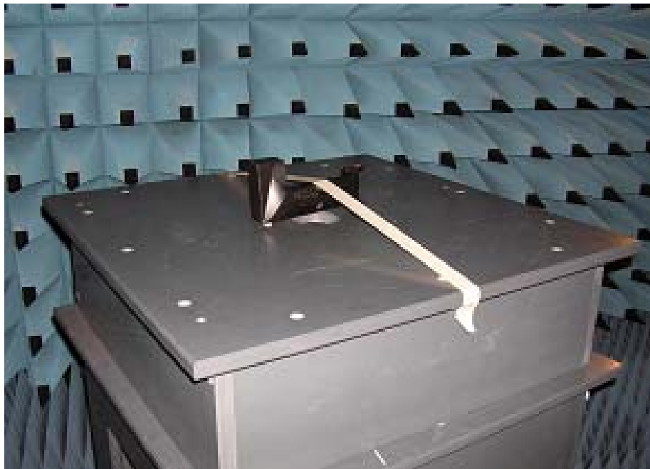
Radiated spurious emission 1-26 GHz
