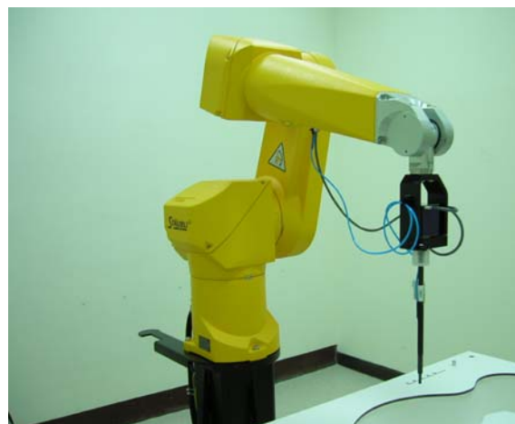
Fig. 5.2 Probe Setup on Robot
