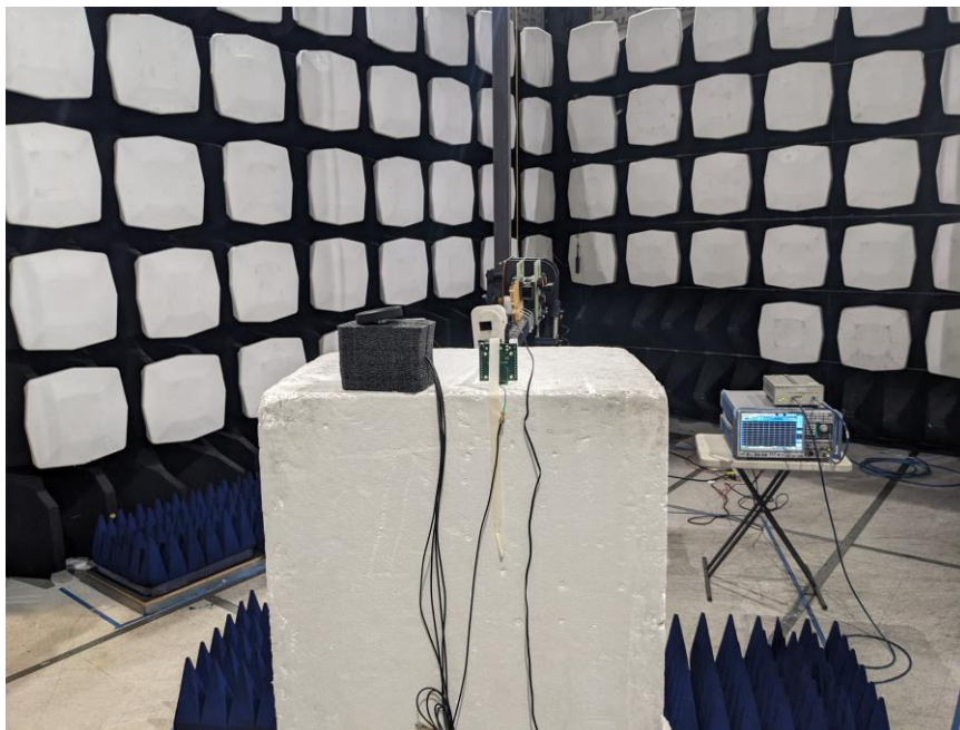
Figure:10– Test Set up – Rear View of the EUT - Radiated Emissions <26 GHz
