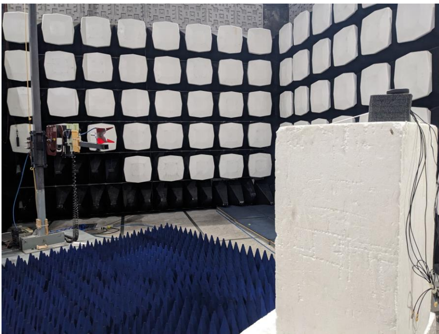
Figure:6– Test Set up – Rear View of the EUT - Radiated Emissions <10 GHz
