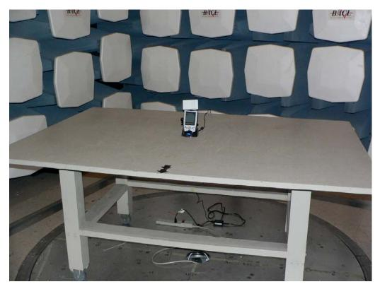
Radiated Emission above 30MHz - Rear View
