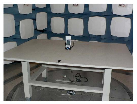
Radiated Emission below 30MHz - Rear View
