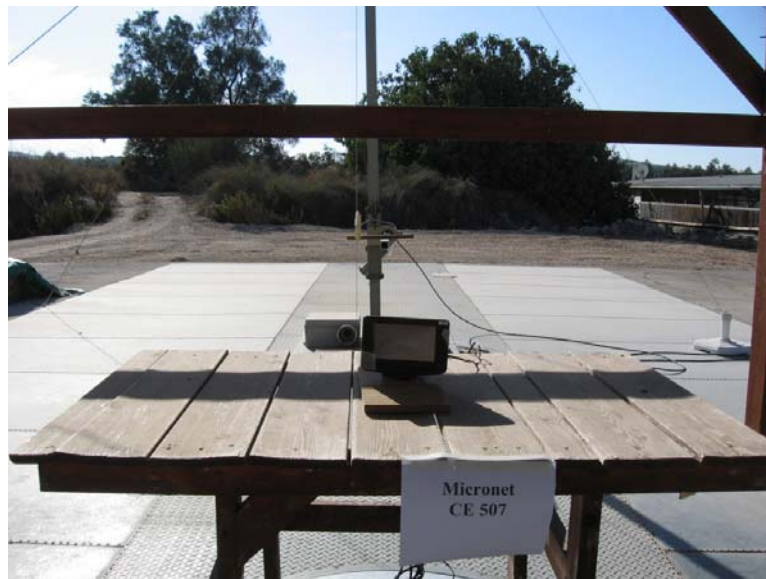
Figure 5. Radiated Emission Test
