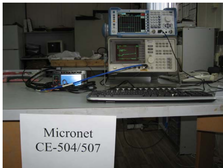
Figure 6. Conducted Emission from Antenna Port Tests
