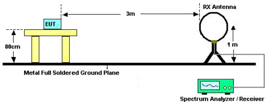
For radiated emissions from 30MHz to 1GHz
