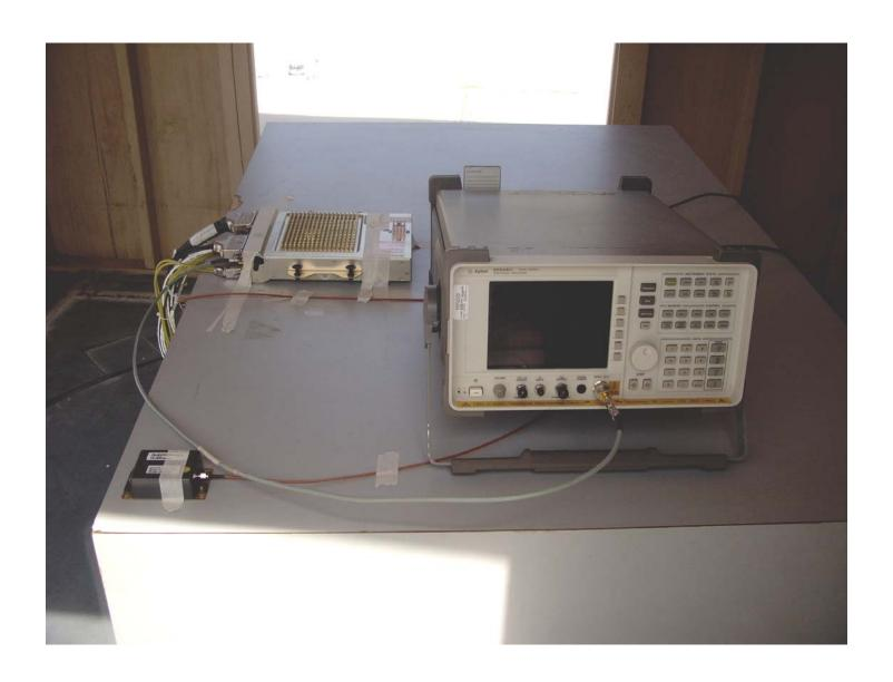
Conducted Emissions at Antenna Terminal Setup
