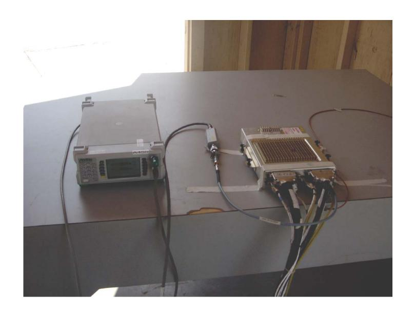
Maximum Peak Output Power Measurement Setup
