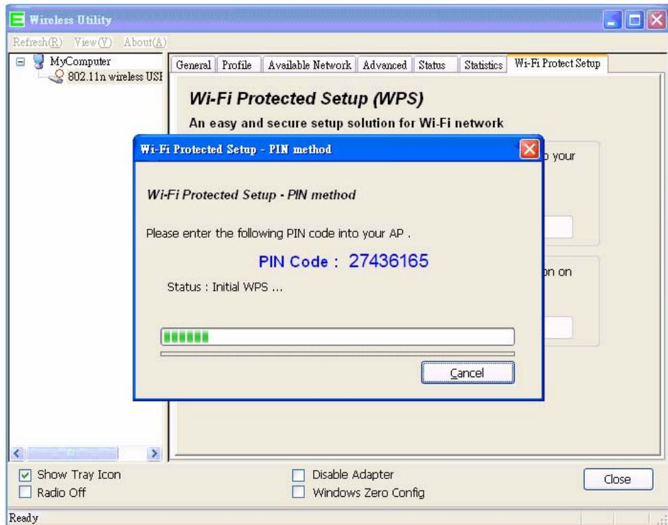
(2.) Open menu “**Wi-Fi Protected Setup**” of 11N Mini Broadband Router , input the PIN number from the wireless card then click **Start PIN**.
