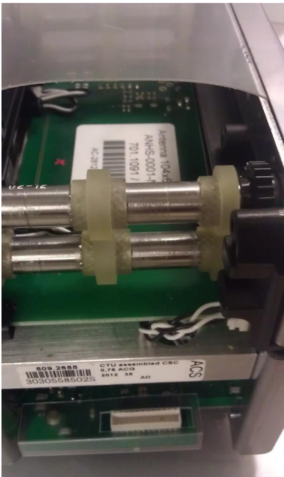
Card dispenser: Close view onto the dispensing part and the RFID antenna
