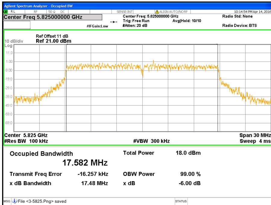
**CH Low (IEEE 802.11ac VHT40 Mode / Band 3 / Chain 0)**
