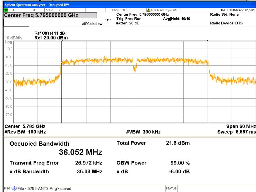
**CH Low (IEEE 802.11ac VHT80 Mode / Band 3 / Chain 0)**
