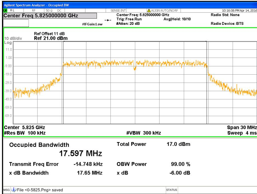
**CH Low (IEEE 802.11ac VHT20 Mode / Band 3 / Chain 1)**
