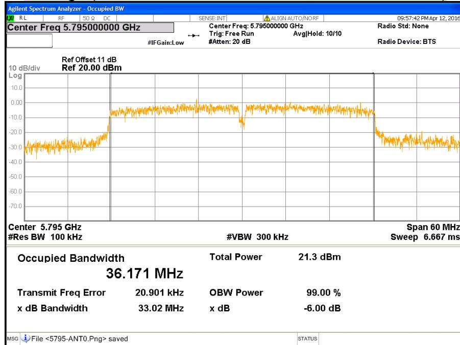
**CH Low (IEEE 802.11ac VHT40 Mode / Band 3 / Chain 1)**
