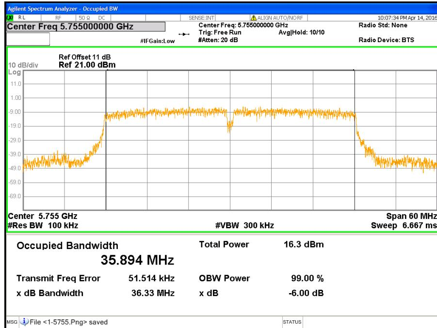
**CH High (IEEE 802.11ac VHT40 Mode / Band 3 / Chain 1)**
