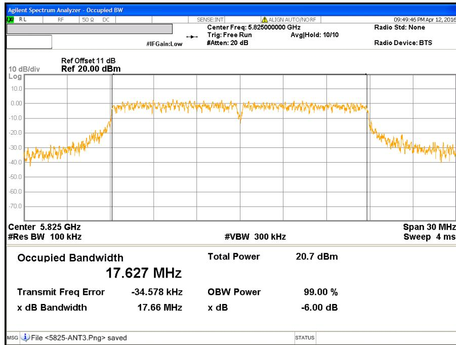
**CH Low (IEEE 802.11ac VHT40 Mode / Band 3 / Chain 0)**
