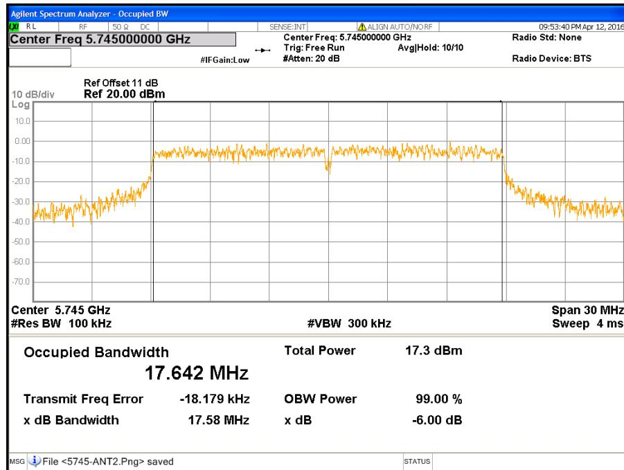
**CH Middle (IEEE 802.11ac VHT20 Mode / Band 3 / Chain 2)**
