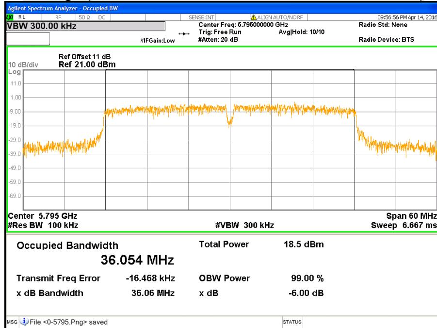
**CH Low (IEEE 802.11ac VHT40 Mode / Band 3 / Chain 1)**
