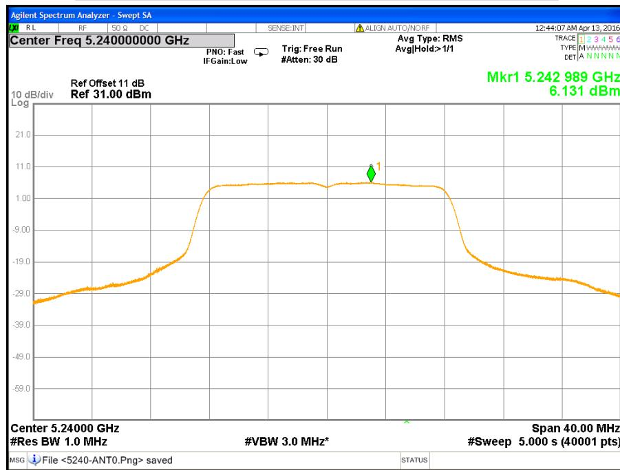
**CH Low (IEEE 802.11a Mode / Band 1 / Chain 1)**
