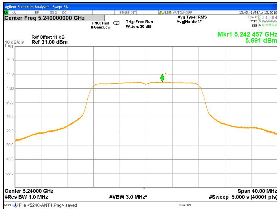
**CH Low (IEEE 802.11a Mode / Band 1 / Chain 2)**
