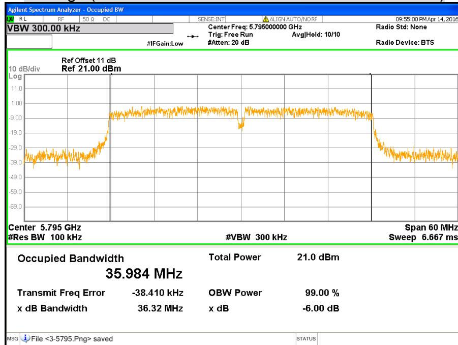
**CH Low (IEEE 802.11ac VHT80 Mode / Band 3 / Chain 0)**
