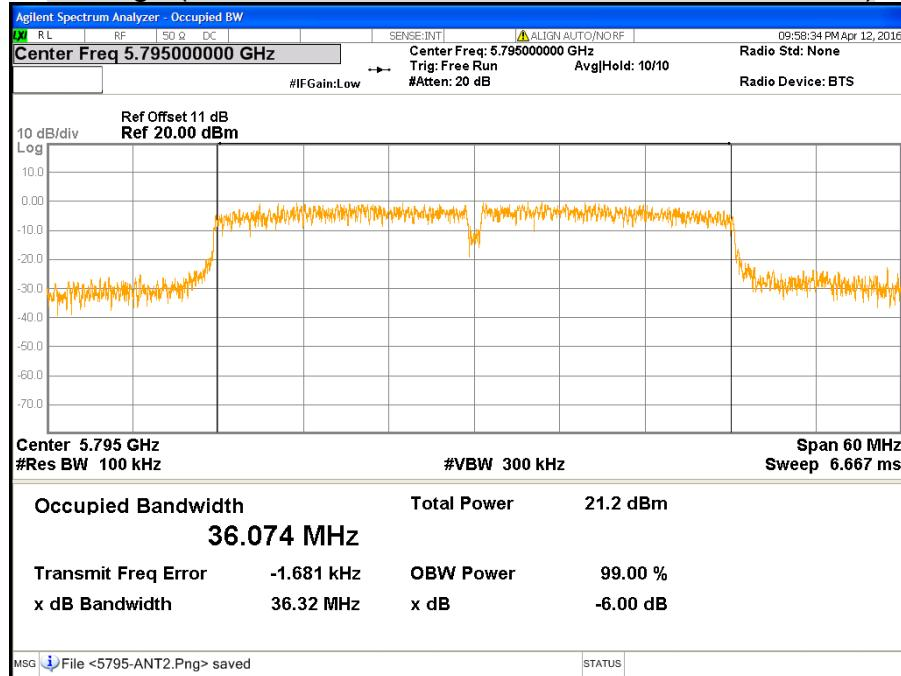
**CH Low (IEEE 802.11ac VHT40 Mode / Band 3 / Chain 3)**
