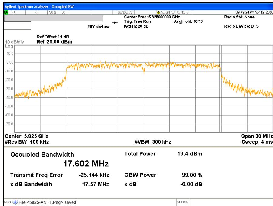
**CH Low (IEEE 802.11ac VHT20 Mode / Band 3 / Chain 2)**
