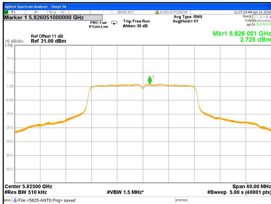
**CH Low (IEEE 802.11a Mode / Band 3 / Chain 1)**
