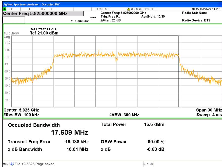
**CH Low (IEEE 802.11ac VHT20 Mode / Band 3 / Chain 3)**
