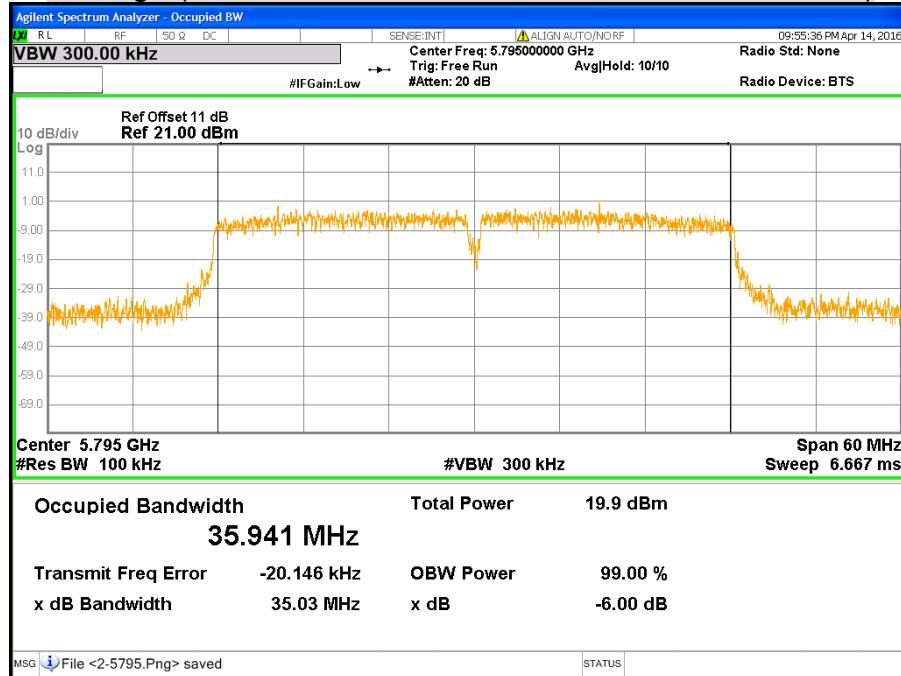
**CH Low (IEEE 802.11ac VHT40 Mode / Band 3 / Chain 3)**
