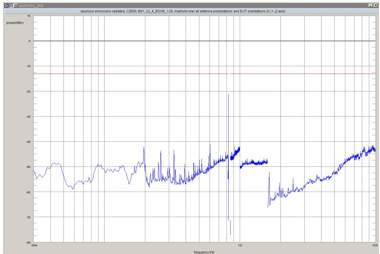
**Test: 22.4; Frequency Band = 850, Mode = EDGE, Channel = 190, Frequency = 836.6MHz**
