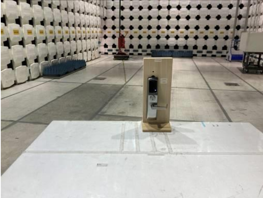
13.56 MHz RFID Test Setup (NTT – Touch Screen), 30 - 1000 MHz
