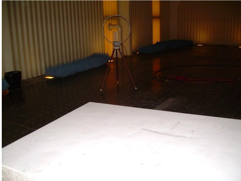
Photograph 10: Reference Photo of Test Setup for Emissions Below 30 MHz
