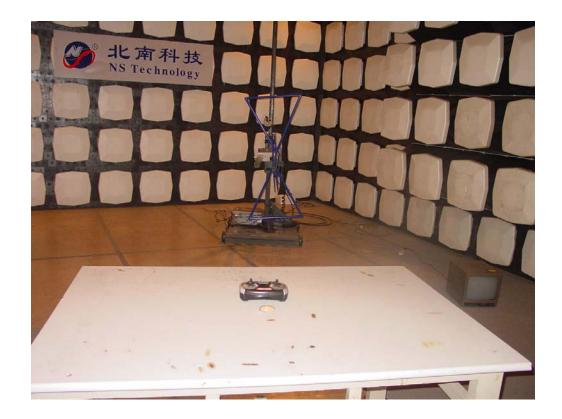
1.2.Set-up for radiated emission test(ABOVE 1GHz)
