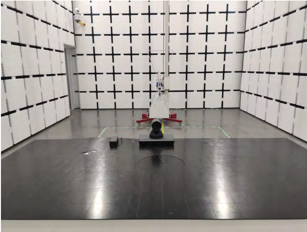
Spurious Radiation Emissions Test (<1G)
