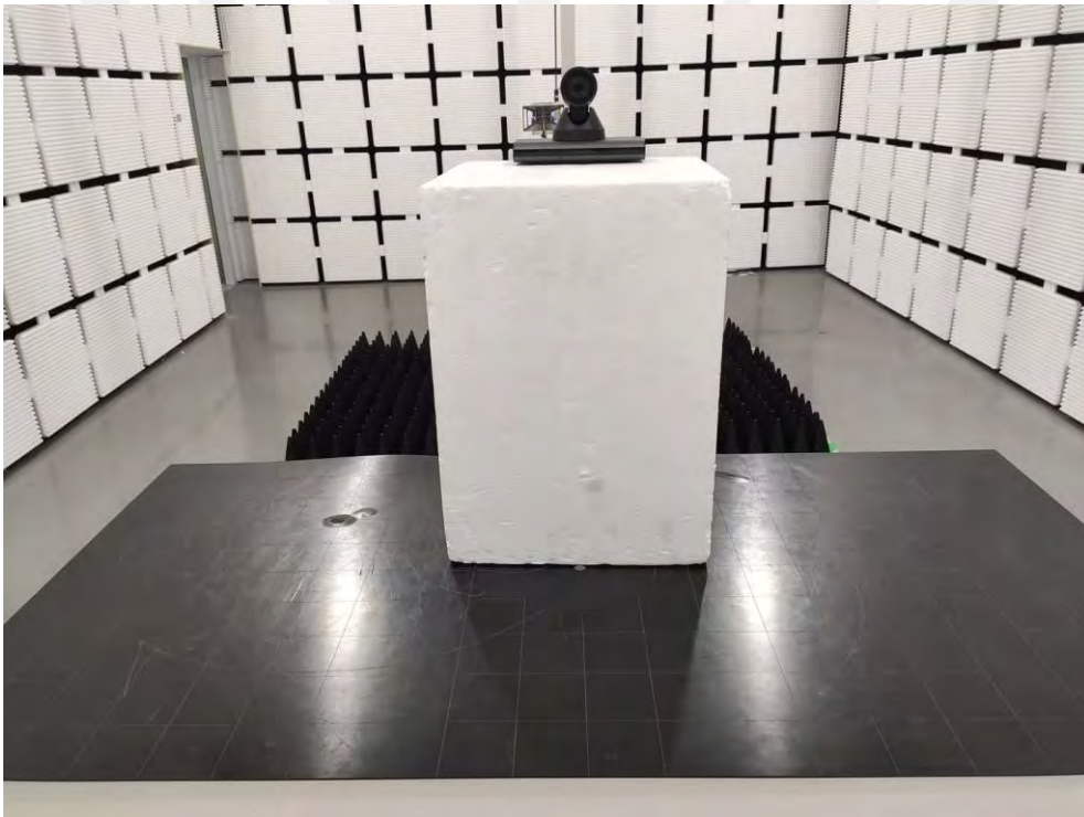
Spurious Radiation Emissions Test (> 1G)
