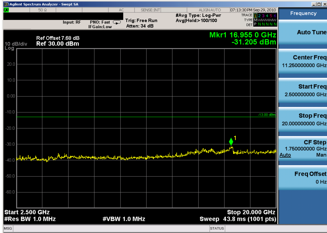
Plot 7-13. Conducted Spurious Plot (PCS CDMA Mode – Ch. 25)
