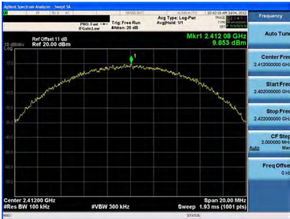
Power Spectral Density (802.11b-CH 6)
