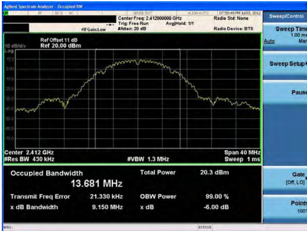
6dB Bandwidth plot (802.11b-CH 6)
