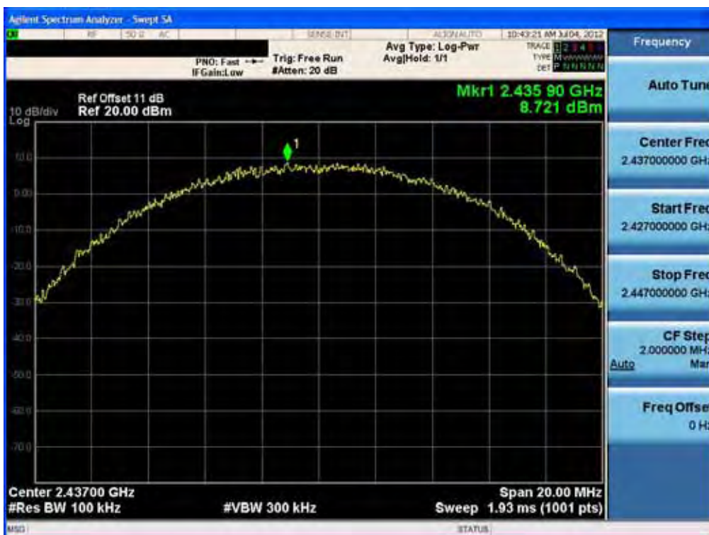
Power Spectral Density (802.11b-CH 6)
