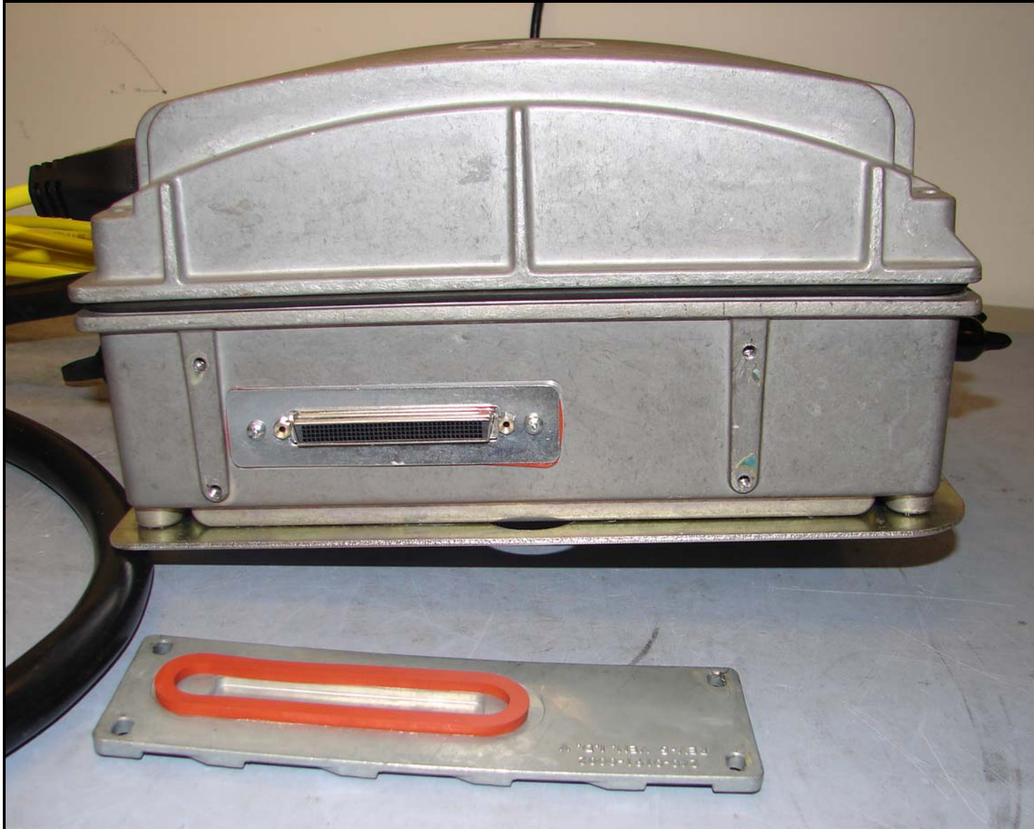
Photograph EP-6: External Photo of CT OTP – View of Expansion Port Side with Expansion Side exposed
