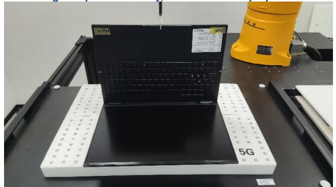
Testing Setup for Extremity, Front Side of Laptop at 2 mm
