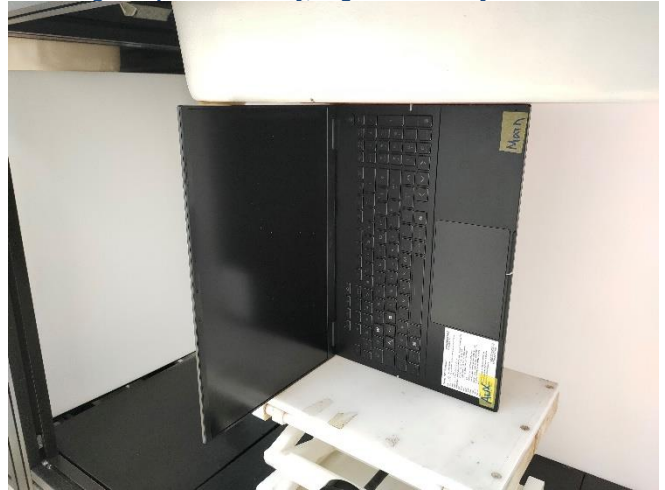
Testing Setup for Extremity, Right Side of keyboard at 0 mm
