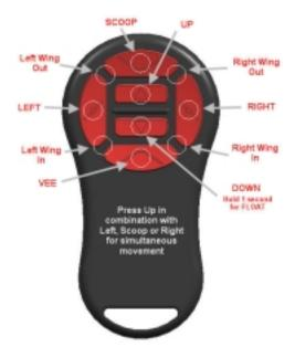
Pressing **SCOOP** button A will bring the plow into a scoop position by automatically positioning both wings forward.
