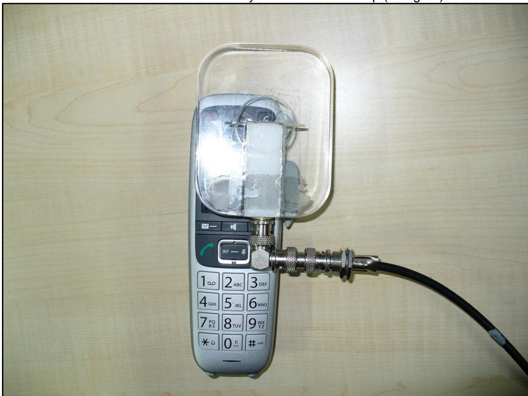
Photo 4: Radial field intensity measurement set-up (0 degree)
