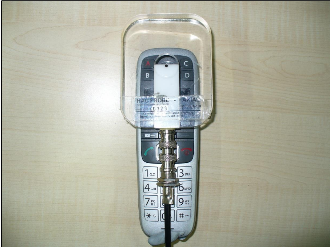
Photo 4: Radial field intensity measurement set-up (0 degree)
