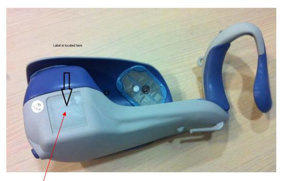
The label with FCC ID:TVF-H200W-RFSO will be located here. The part 15 statement required by FCC rules, paragraph 15.19 (a)(3), is inserted into the Users\_guide\_21560, page 12, provided to the user together with each unit.
