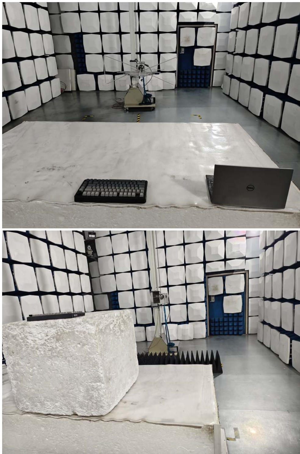
Radiated emission test view
