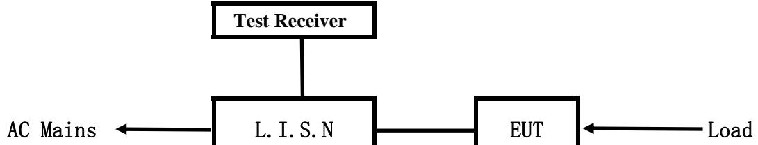
EUT: Equipment Under Test
