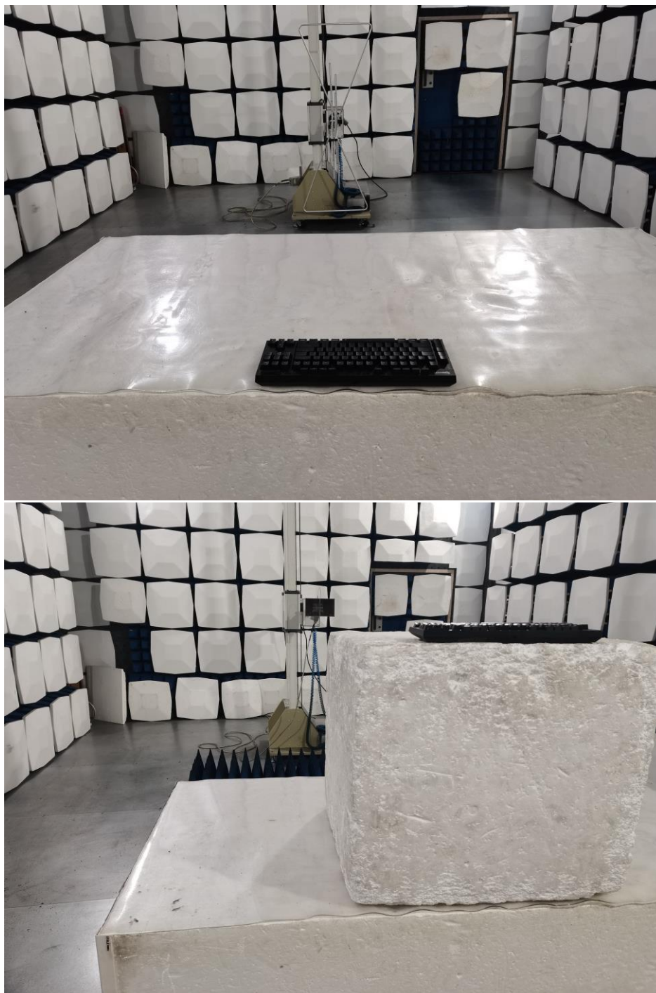
Radiated emission test view
