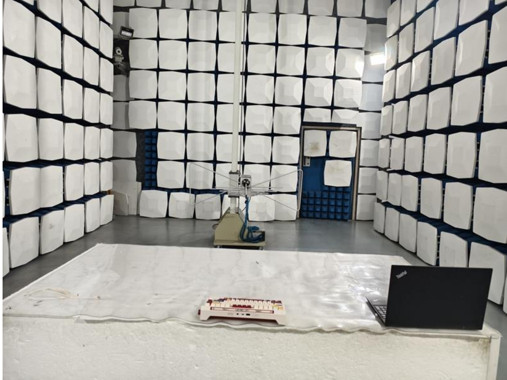
Radiated Emission Test Setup:
