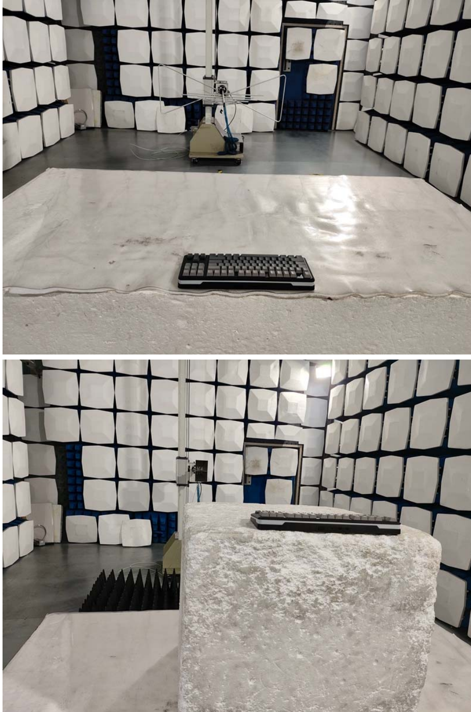
Radiated emission test view
