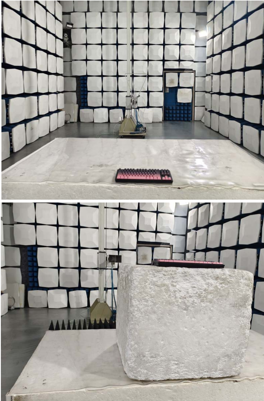
Radiated emission test view
