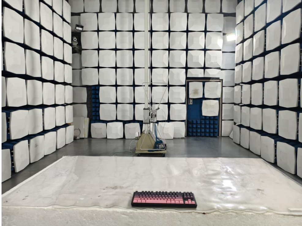
Radiated Emission Test Setup:
