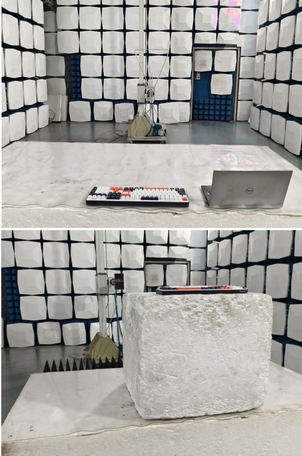
Radiated emission test view
