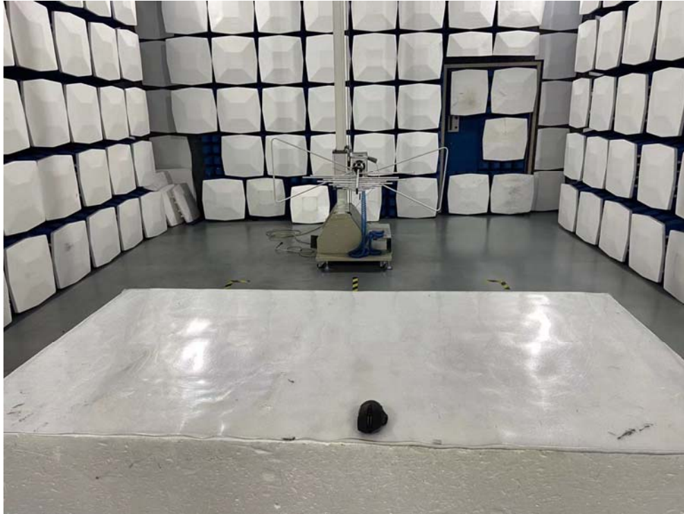
Radiated emission test view
