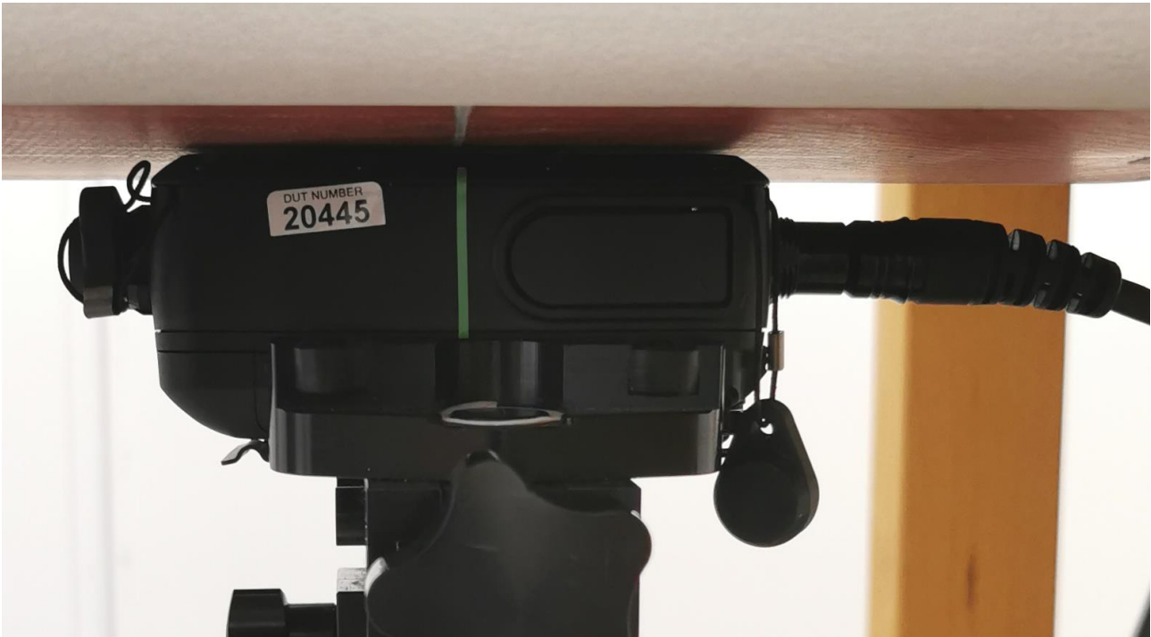
Figure 7 Front side of the DUT against the phantom, 0mm separation distance
