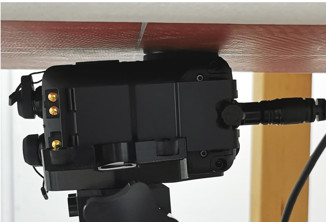
Figure 10 Right side of the DUT against the phantom, 0mm separation distance
