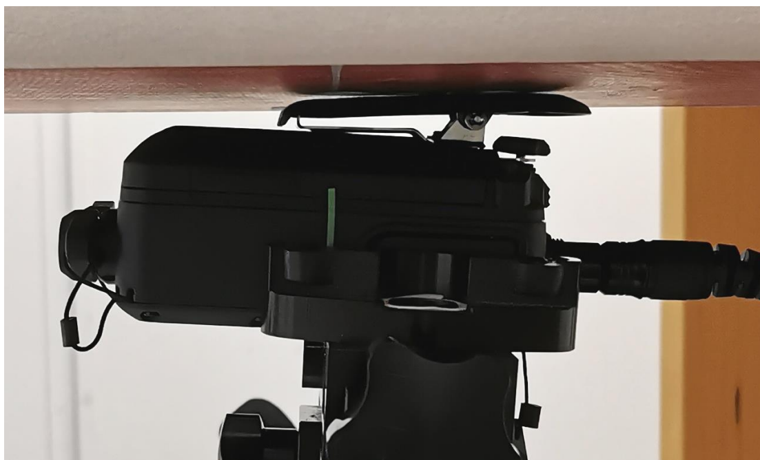
Figure 13 Spot Check measurement with different clip, back side of the DUT against the phantom, 0mm separation distance
