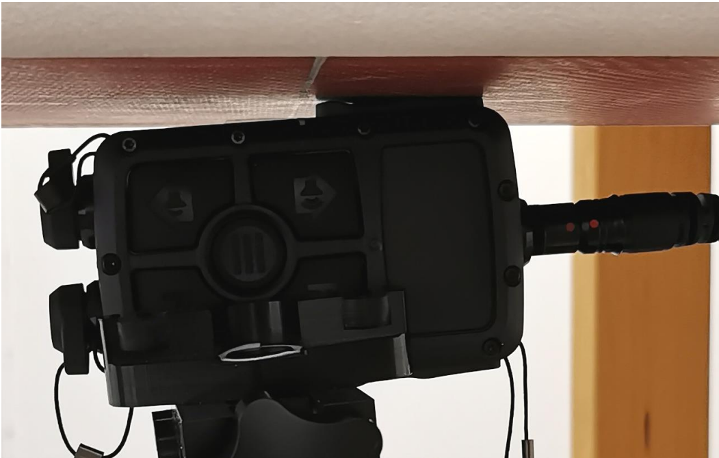
Figure 9 Left side of the DUT against the phantom, 0mm separation distance
