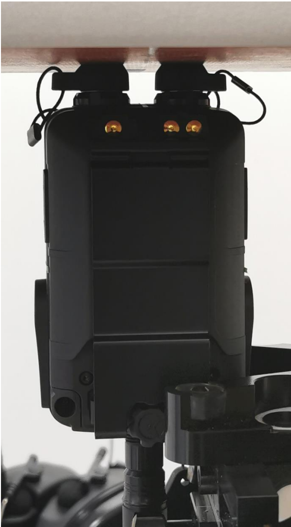
Figure 11 Bottom side of the DUT against the phantom, 0mm separation distance
