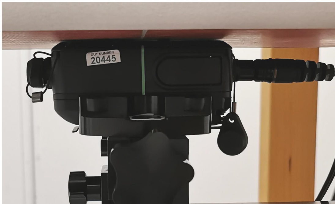
Figure 12 Spot Check Measurement with earplugs, front side of the DUT against the phantom, 0mm separation distance
