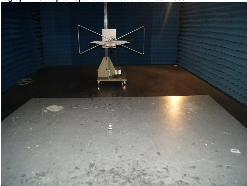
Photograph 2: Set-up for Spurious Emissions for 30 - 1000MHz
